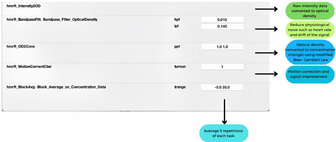
**Figure 8: Processing stream to analyze raw fNIRS data during standing balance in Homer3.**
