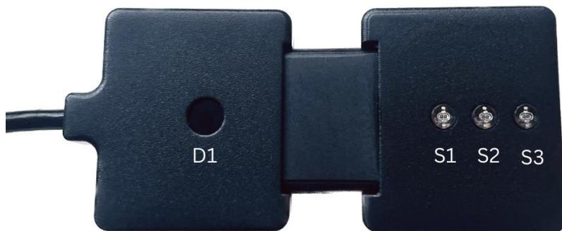
**Figure 6: Close-up of source-detector pairings on the Portalite fNIRS system. D1: Detector 1, S1: Source 1 (30mm), S2: Source 2 (35mm), S3: Source 3 (40mm).**
