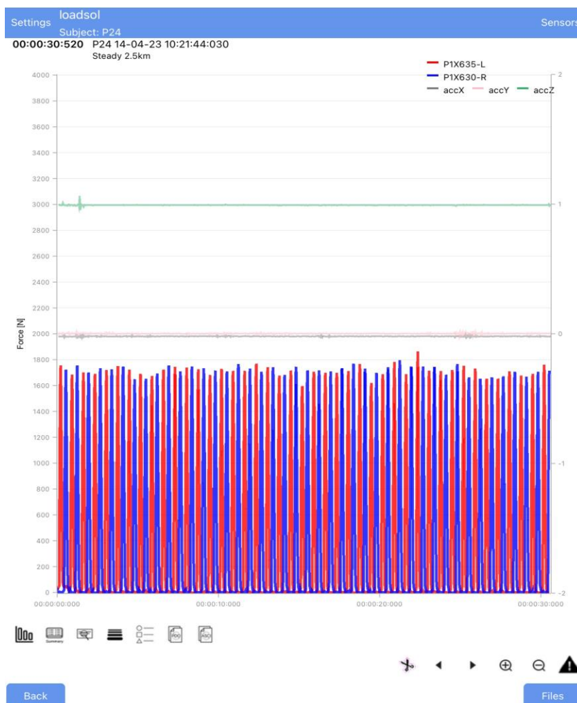
Figure 4: Screenshot of Loadsol Kinetic Data Bluetooth Stream to Apple iPad During Collection; The y axis is force in newtons and the x axis is time in seconds. The lines represent the force reading for each contact (red = left, blue = right).
