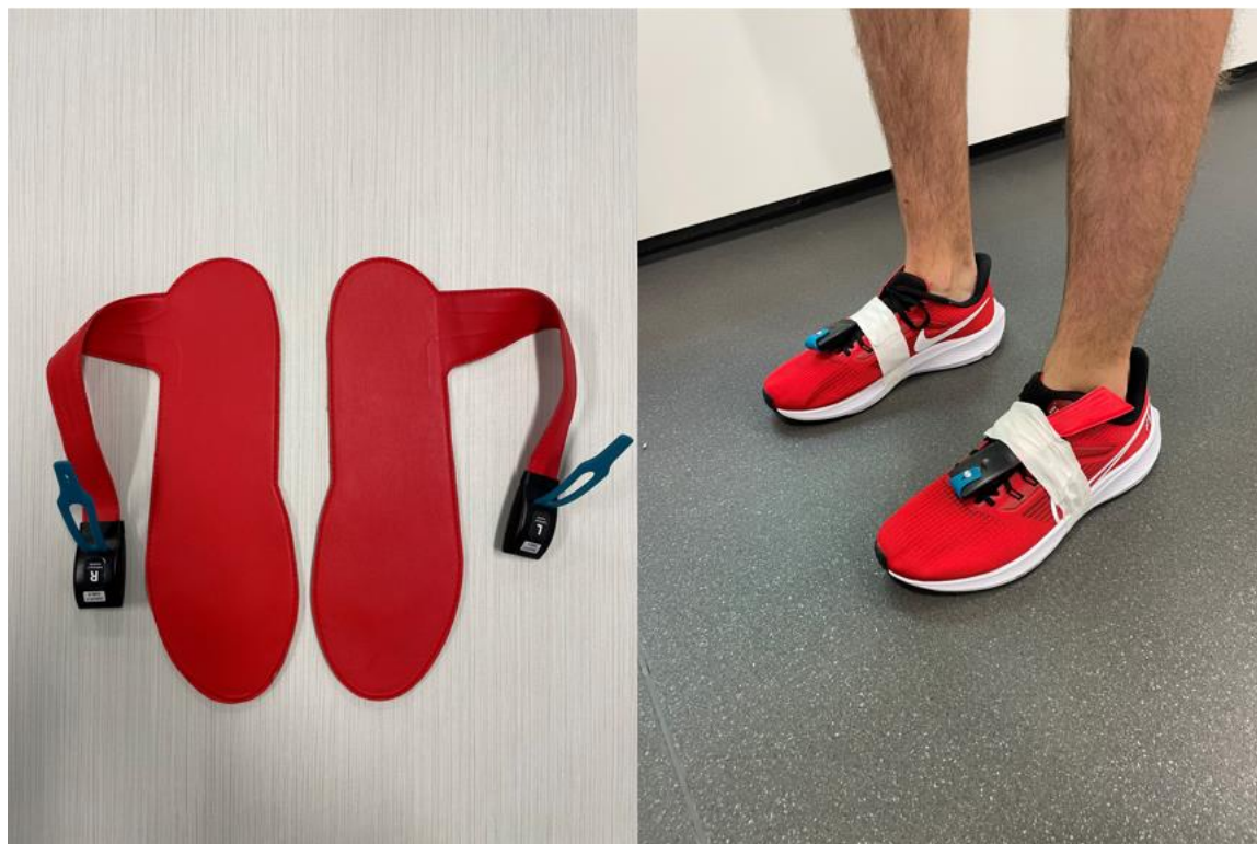
Figure 3: Image of Loadsols; The Left image is the Loadsols outside of the shoes to see the insole, strap, and electronics box. The right image is of the Loadsols in the participants shoe, replacing the insoles, strapped to the shoelaces, and the strap taped around the shoe to ensure it did not detach.
