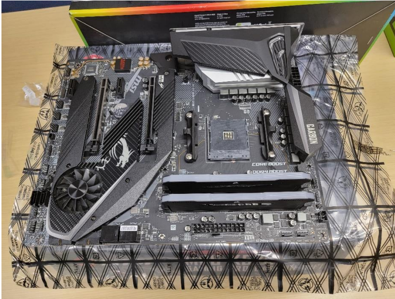
Figure 3-17 Motherboard with RAM Installed for Desktop Build
