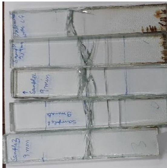
(c) Specimens exposed to fire and tested in flexural while being hot
