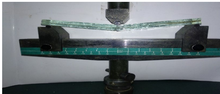
Figure 8. Three-point bending performance assessment of LG specimens.
