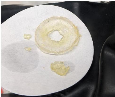
**Figure 3.27. Digital image of the punctured P-91 polymer after a failed electrochemical experiment.**
