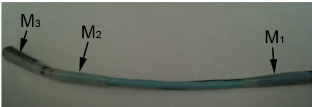
Figure 3.4: Three magnetic tracking sensors ( M_1, M_2, M_3 ) mounted on the distal part of a steerable catheter and fixed using heat-shrink tubes.
