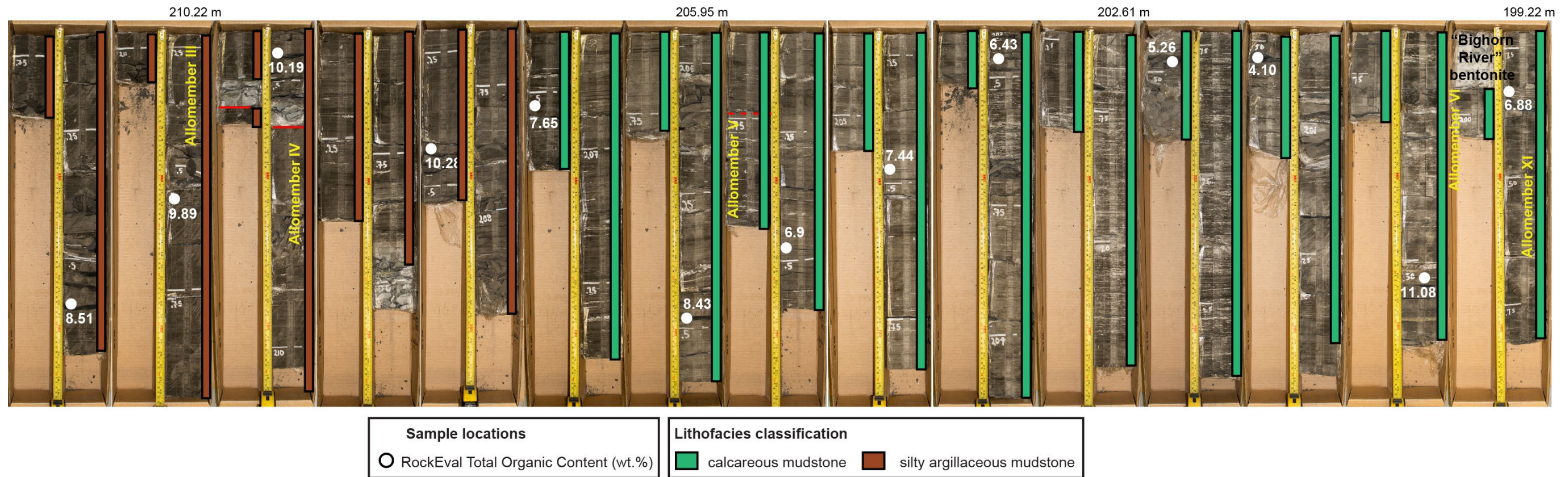
Figure 8:10: Core photo of TOC results from samples collected from silty argillaceous mudstone and calcareous mudstone in well 141/07-34-035-01W2 and TOC results. The TOC varies between 4.10 and 11.08 wt.%.
