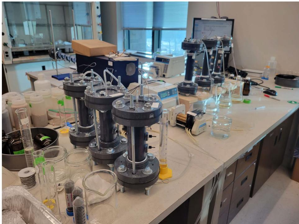
**Figure A. 2** Leaching columns (right) and humidity cells (left) during SIP measurement
