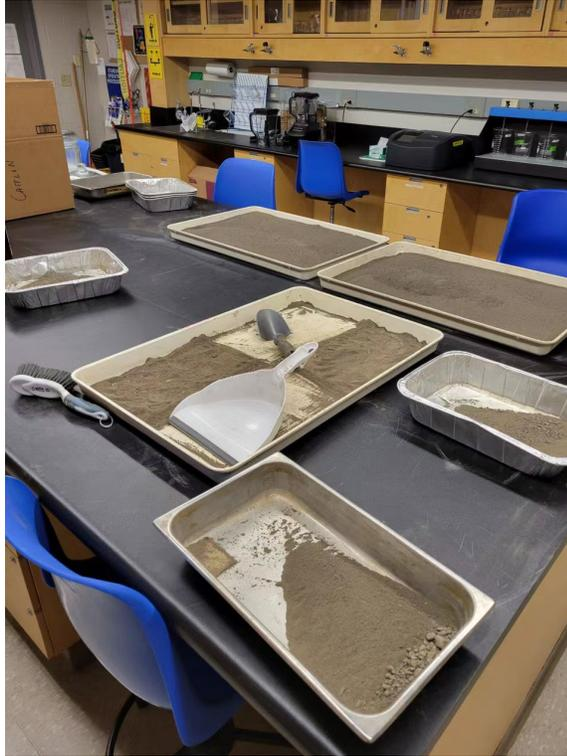
**Figure D. 2** Sample preparation – quartering and mixing (1)
