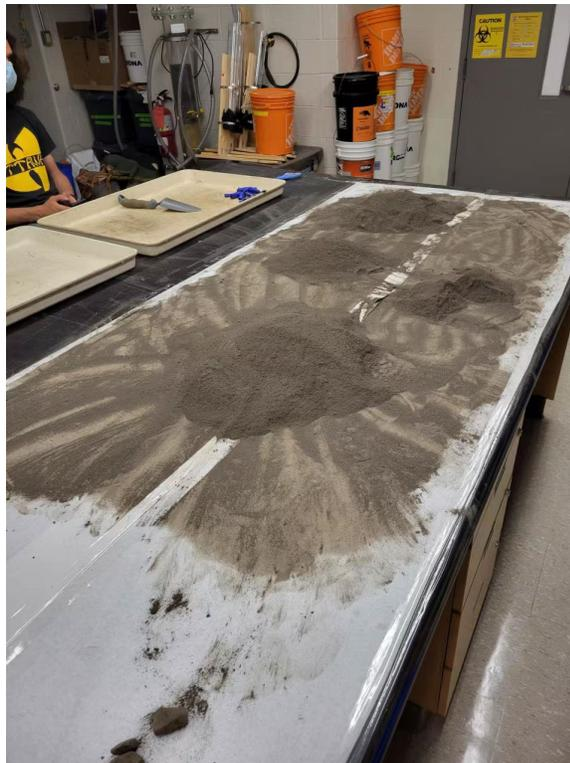
**Figure D. 3** Sample preparation – quartering and mixing (2)
