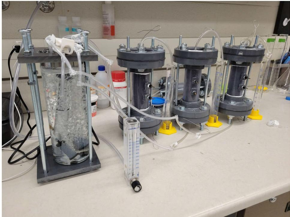
**Figure A. 4** Humidifier (left) and humidity cells (right) during humid air injection period
