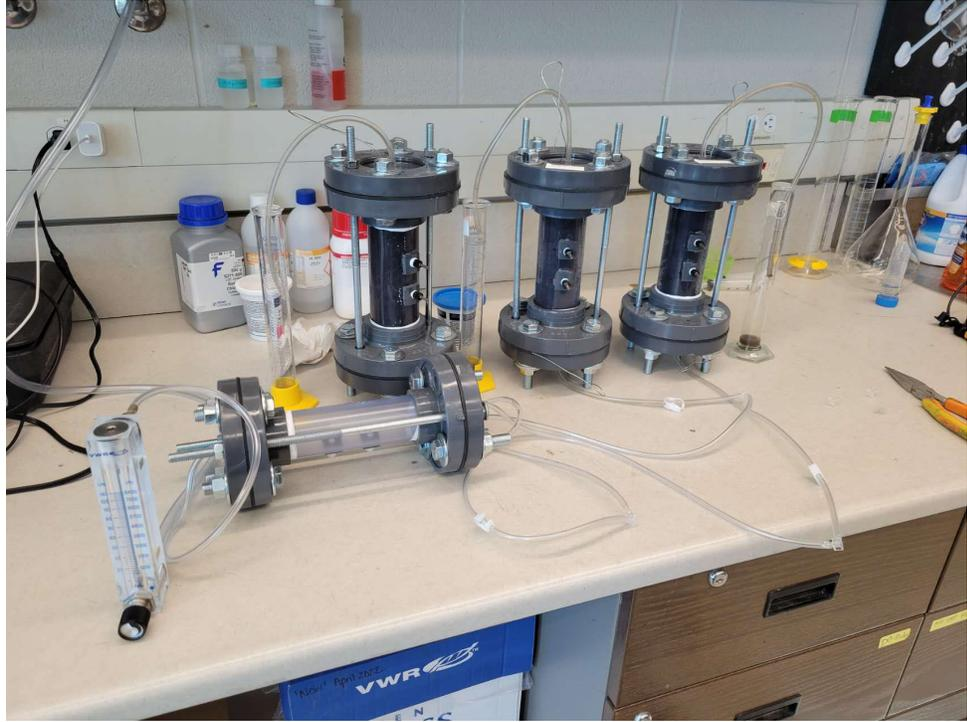
**Figure A. 3** Dry air column (left) and humidity cells (right) during dry air injection period
