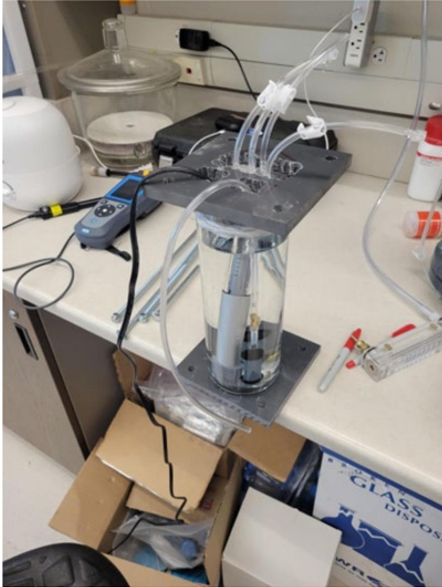
**Figure A. 5** Construction of humidifier
