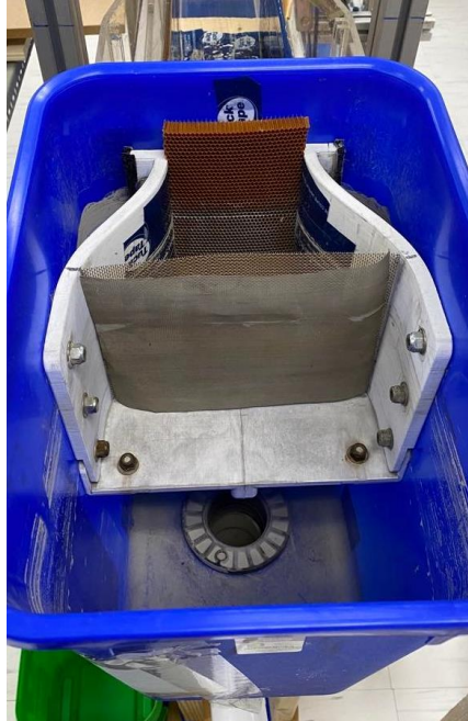
Figure 97: Final inlet configuration with two stages of flow conditioning and curved contraction section.
