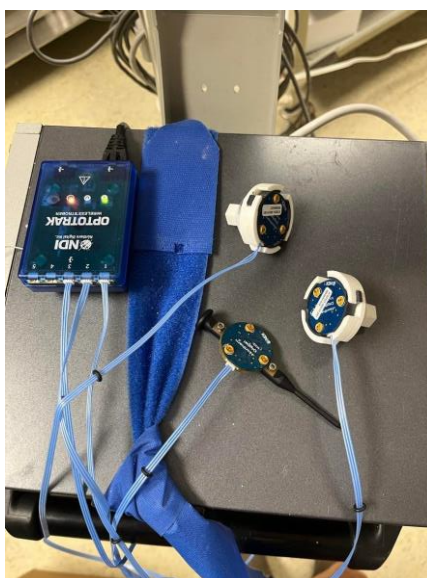
Figure 3.5: Infrared emitting trackers (encased in white) that mount onto bone screws and the stylus for the Optotrak Certus
