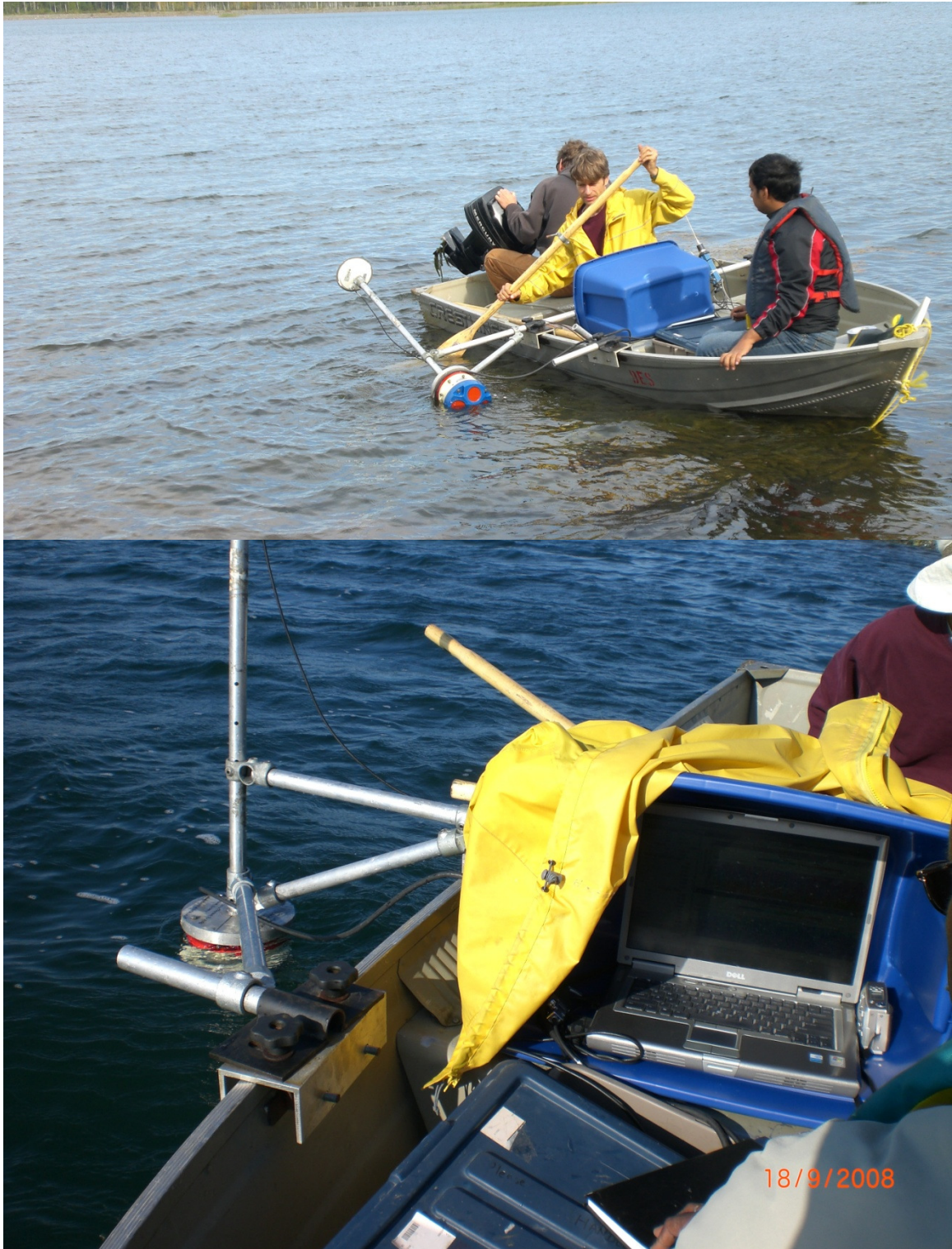
Figure IV-11 Stationary boat data circulation current data collection with ADCP in the middle cell of the tailings pond
