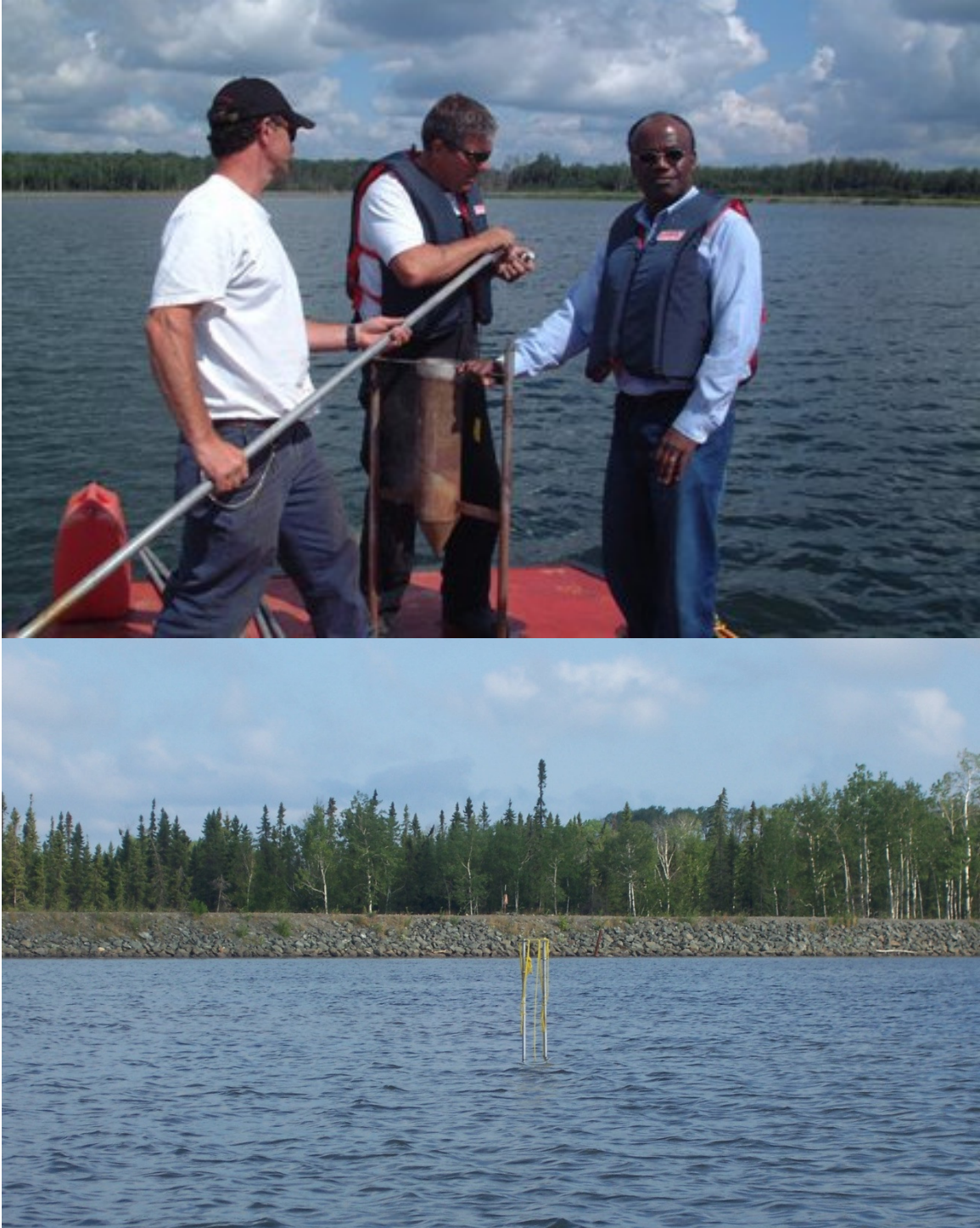
Figure IV-6 Deployment of sediment traps by professional divers under supervision of Prof. Ernest K. Yanful (on right) and a properly installed sediment trap
