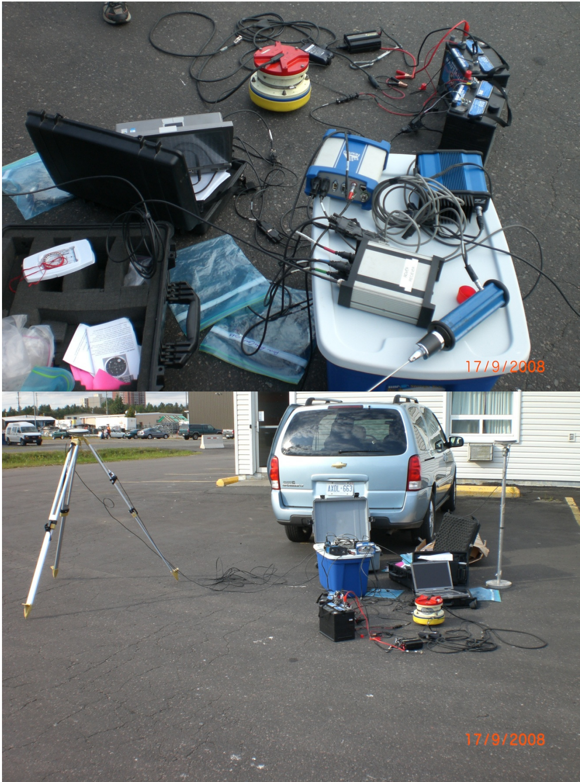
Figure IV-9 Testing of ADCP and peripherals prior to deployment in the tailings pond
