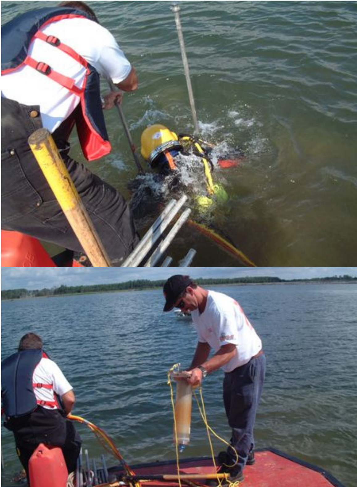
Figure IV-5 Deployment of sediment traps by professional divers in the tailings pond
