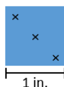
Figure 16: Scaled schematic of a 1 x 1 in. quartz substrate, indicating the spectroscopy probing locations ('x').
