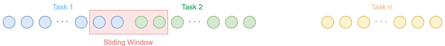
Figure 4.1: The new proposed setting: Data comes in as a stream and access is defined by a sliding window.
