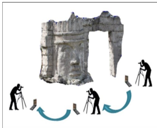
Figure 2: Close-range photogrammetry using a tripod
