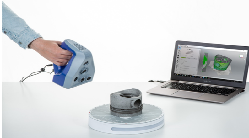
Figure 10: Method to capture images using ASS
