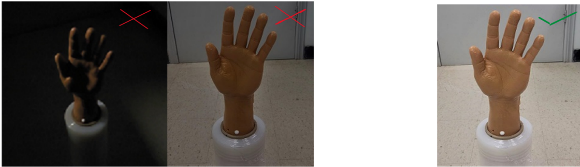
Figure 37: The images on the left are shadowed images without proper lighting, while the image on the right is an image with homogenous lighting and is considered the correct image for photogrammetry.
