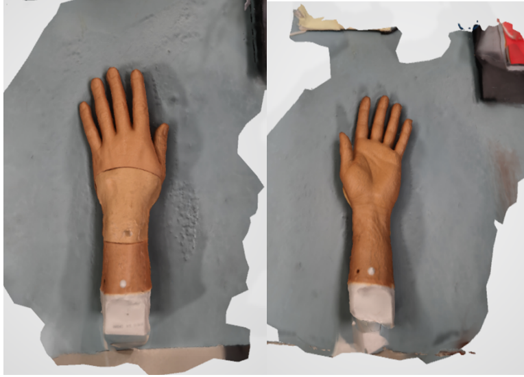
Figure 54:3D model of a) dorsal side of hand prosthetic b)palmer side of hand prosthetic using KIRI Engine
