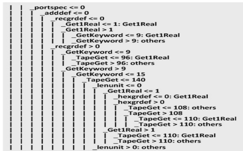
Figure 27: The C4.5 decision tree model for the function ‘Get1Real’ of the Space program from failed traces of mutants by using one-against-all approach.
