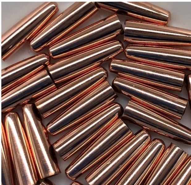
**Figure 3.1: O-free, P-doped copper electrodes.**
