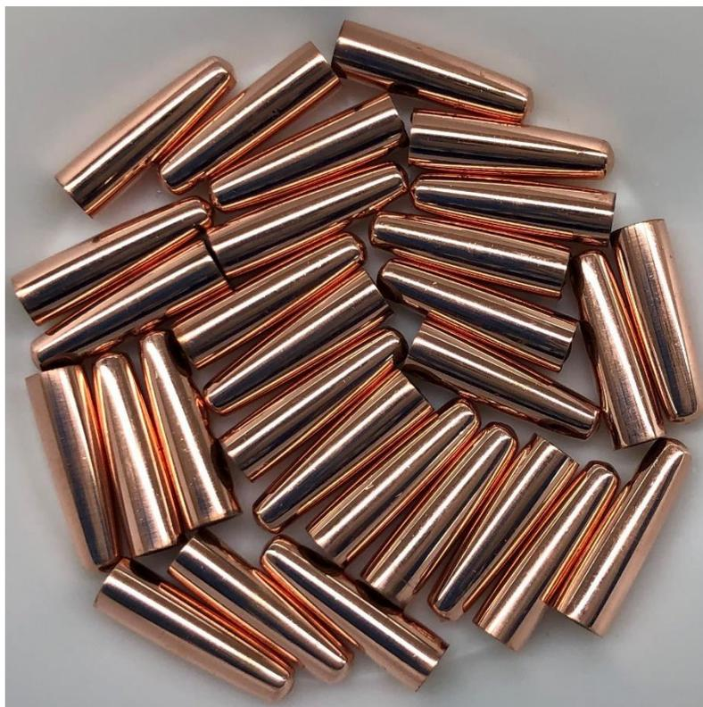
**Figure 2.1: O-free and P-doped copper electrodes.**
