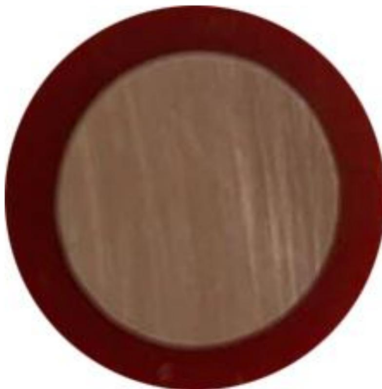
**Figure 2.2: O-free and P-doped single copper electrode mounted in epoxy**
