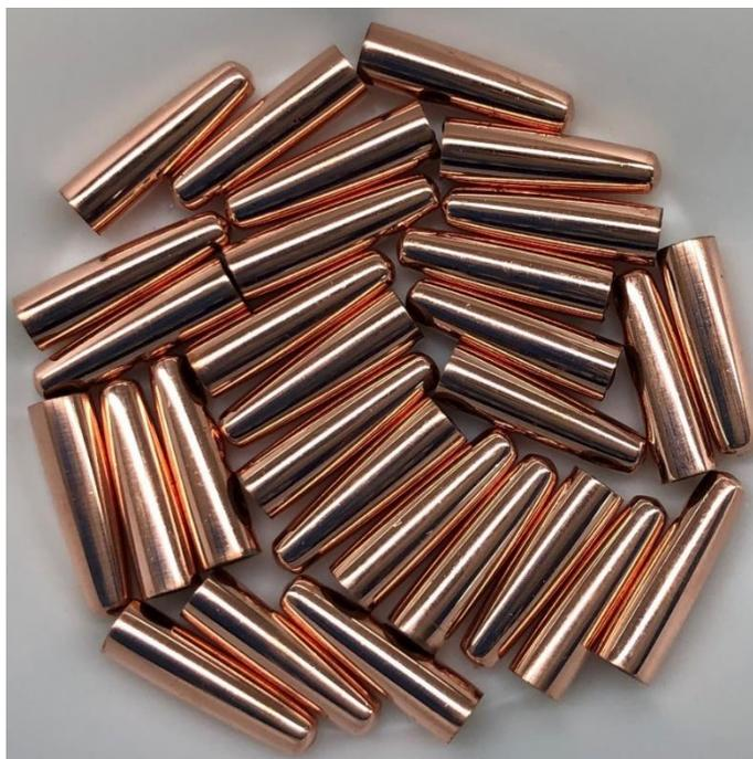
**Figure 5.1: O-free and P-doped copper electrodes.**
