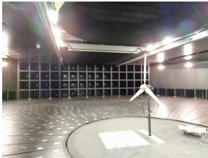
Figure 9 Position of the wind turbine in the WinDEEE Dome test chamber
