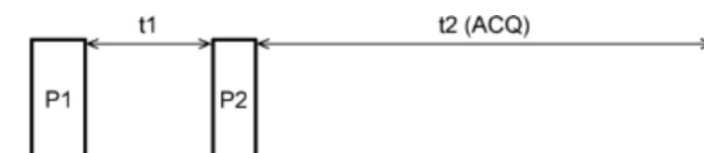
Figure 1-27 Two-pulse sequence and the example of 3Q-MAS in a spin I=5/2 system. 89
