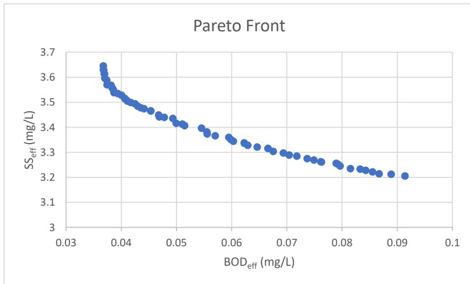
**Figure 5.9 Pareto front of BOD<sub>eff</sub> and SS<sub>eff</sub> for case 2**
