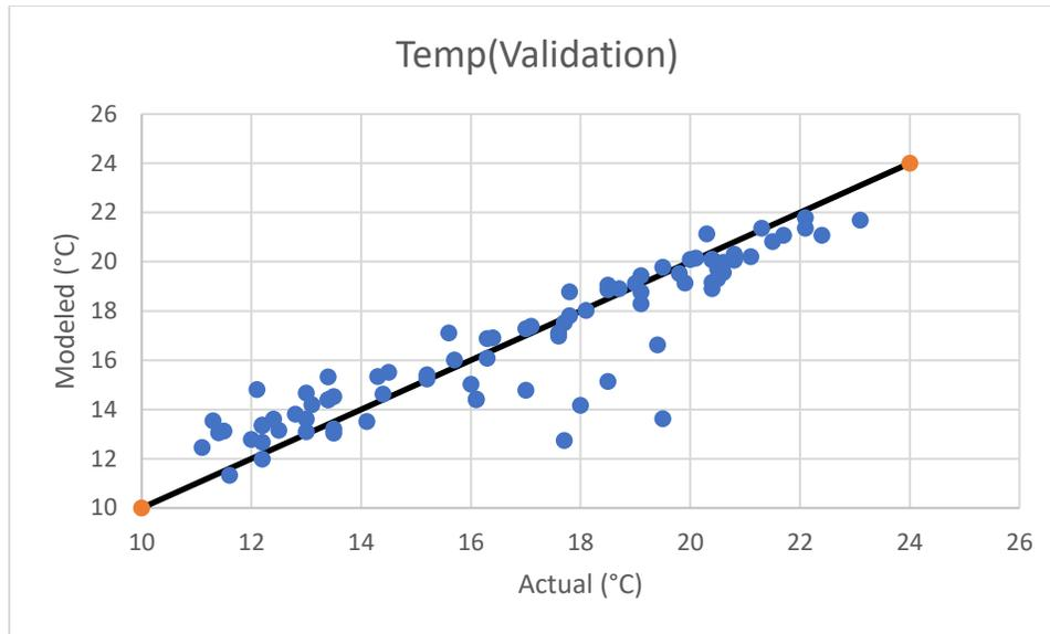
**Figure 4.16 Regression analysis of actual versus ANN-modeled temperature values in effluent stream**
