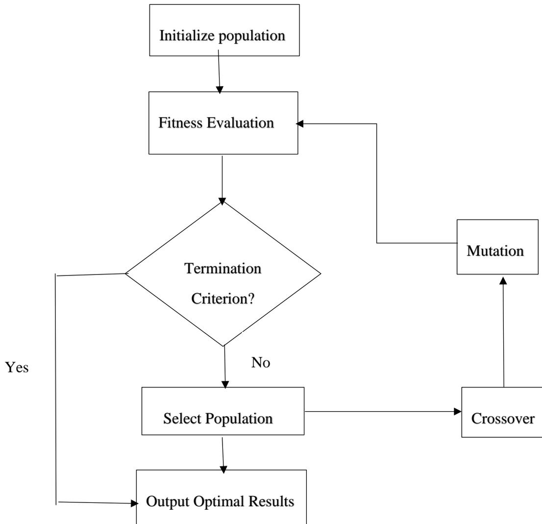
**Figure 5.2: Structure of Genetic Algorithm**
