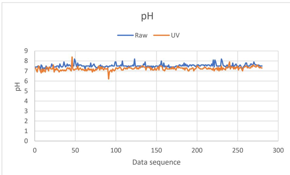
**Figure 3.8 Scatter plot of pH in the influent and effluent stream**
