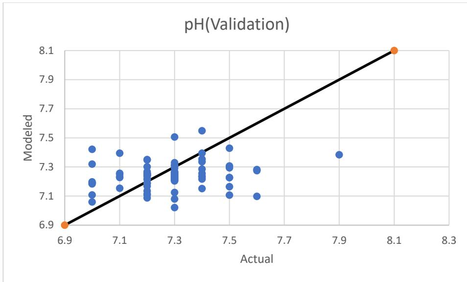
**Figure 4.14 Regression analysis of actual versus ANN-modeled pH values in effluent stream**
