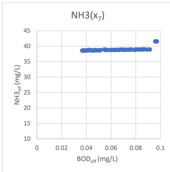
**Figure 5.13 Optimal variation of  $NH3_{inf}$  with  $BOD_{eff}$  for case 2**
