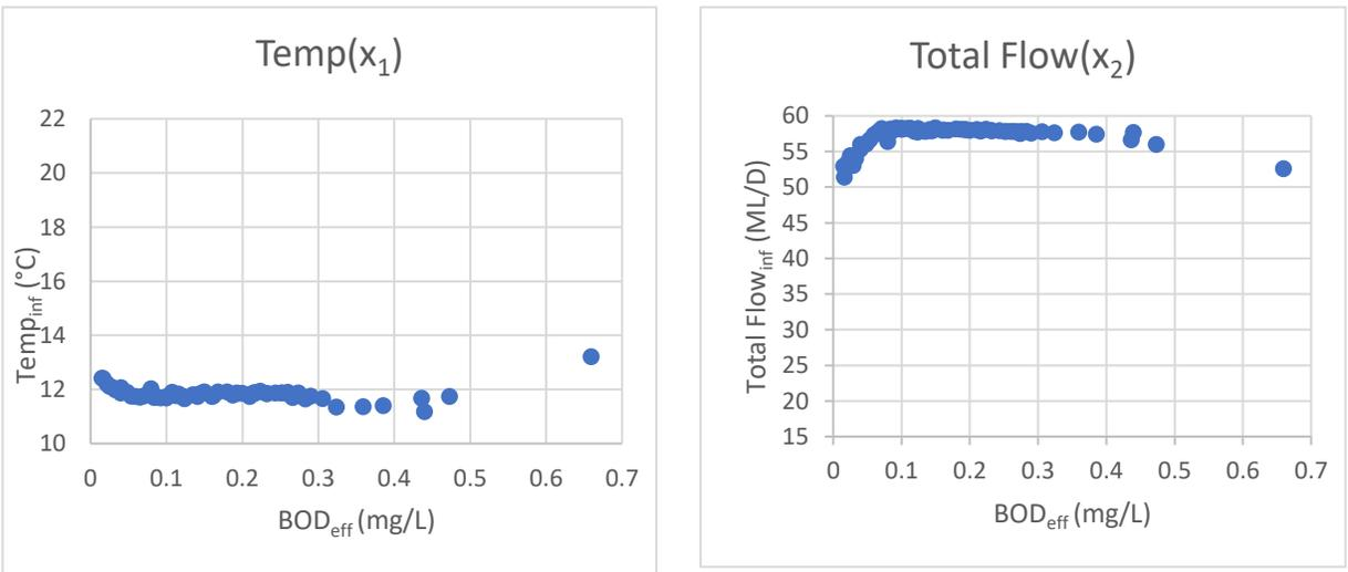
**Figure 5.4 Optimal variation of temp and total flow rate with BOD<sub>eff</sub> for case 1**
