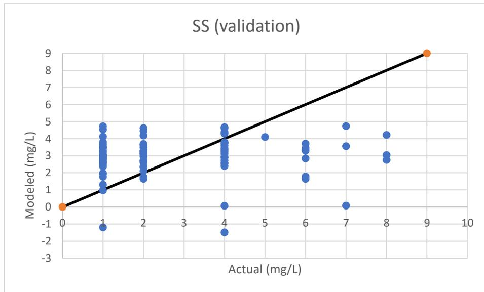
**Figure 4.11 Regression analysis of actual versus ANN-modeled SS concentration in the effluent stream**
