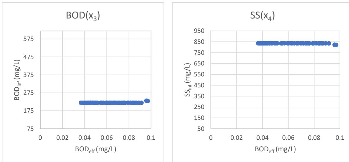
**Figure 5.11 Optimal variation of  $BOD_{inf}$  and  $SS_{inf}$  with  $BOD_{eff}$  for case 2**
