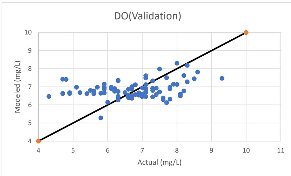
**Figure 4.15 Regression analysis of actual versus ANN-modeled DO concentration in effluent stream**
