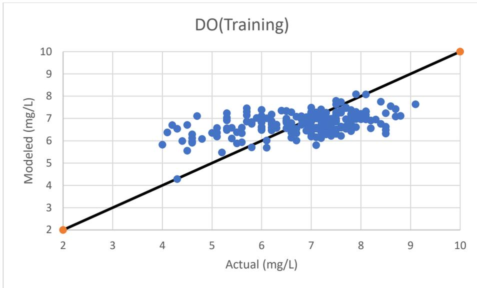
**Figure 4.8 Regression analysis of actual versus ANN-modeled DO concentration in effluent stream**
