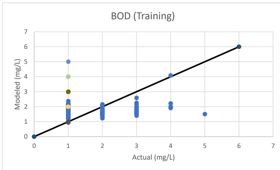
**Figure 4.3 Regression analysis of actual versus ANN-modeled BOD concentration in effluent stream**
