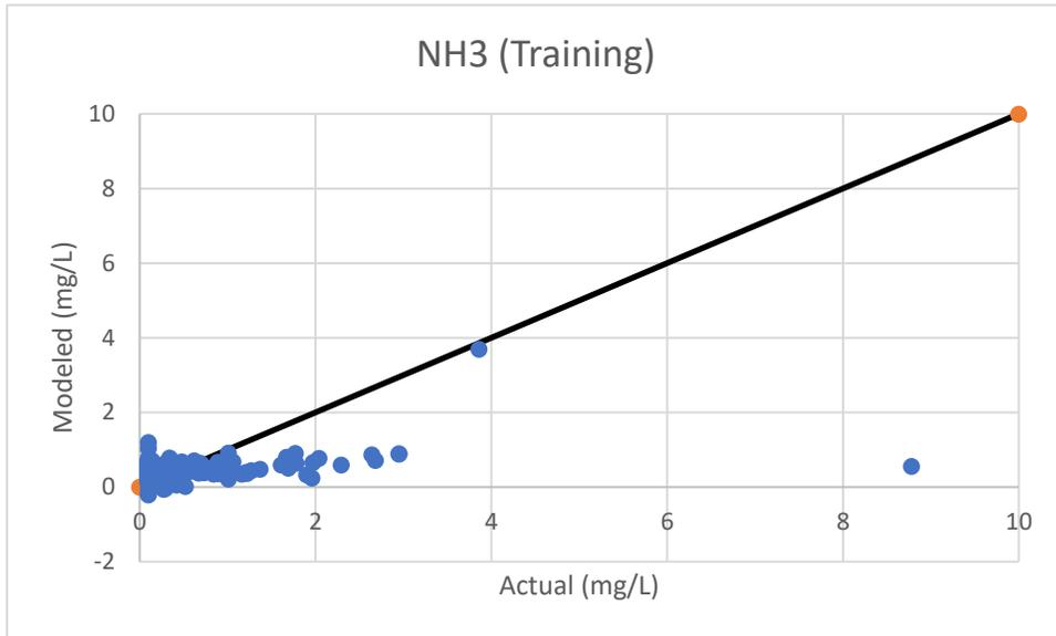
**Figure 4.6 Regression analysis of actual versus ANN-modeled NH3 concentration in effluent stream**
