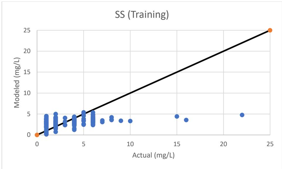
**Figure 4.4 Regression analysis of actual versus ANN-modeled SS concentration in effluent stream**
