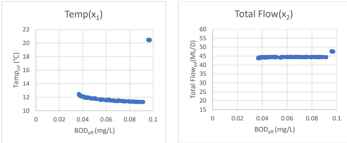
**Figure 5.10 Optimal variation of temp and total flow rate with  $BOD_{eff}$  for case 2**
