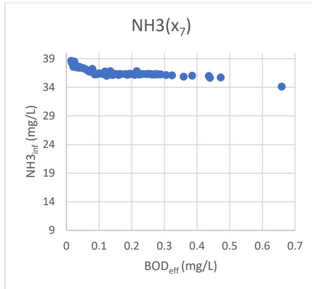
**Figure 5.7 Optimal variation of  $NH3_{inf}$  with  $BOD_{eff}$  for case 1**
