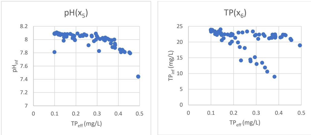
**Figure 5.25 Optimal variation of  $\text{pH}_{\text{inf}}$  and  $\text{TP}_{\text{inf}}$  with  $\text{TP}_{\text{eff}}$  for case 4**
