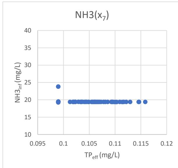
**Figure 5.19 Optimal variation of  $\text{NH}_3_{\text{inf}}$  with  $\text{TP}_{\text{eff}}$  for case 3**
