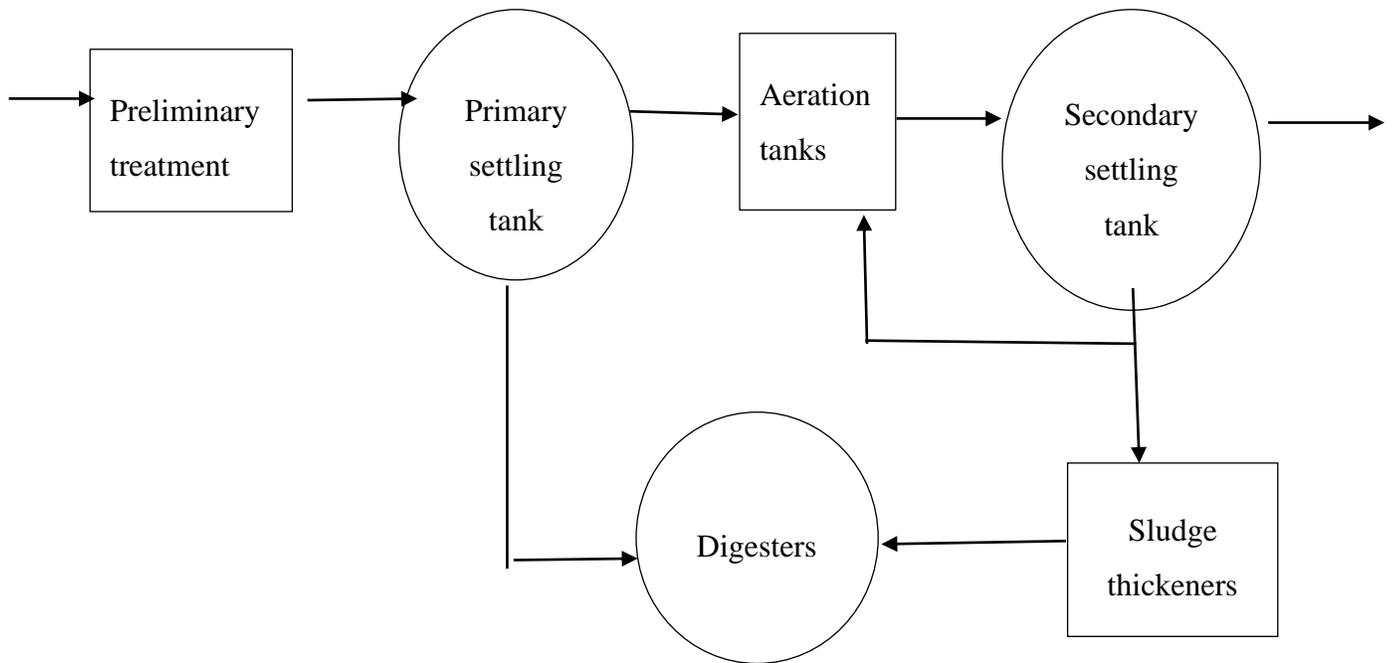
**Figure 3.1 Schematic diagram of WWTP**
