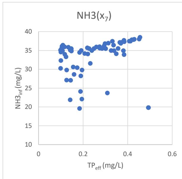
**Figure 5.26 Optimal variation of  $\text{NH}_3_{\text{inf}}$  with  $\text{TP}_{\text{eff}}$  for case 4**
