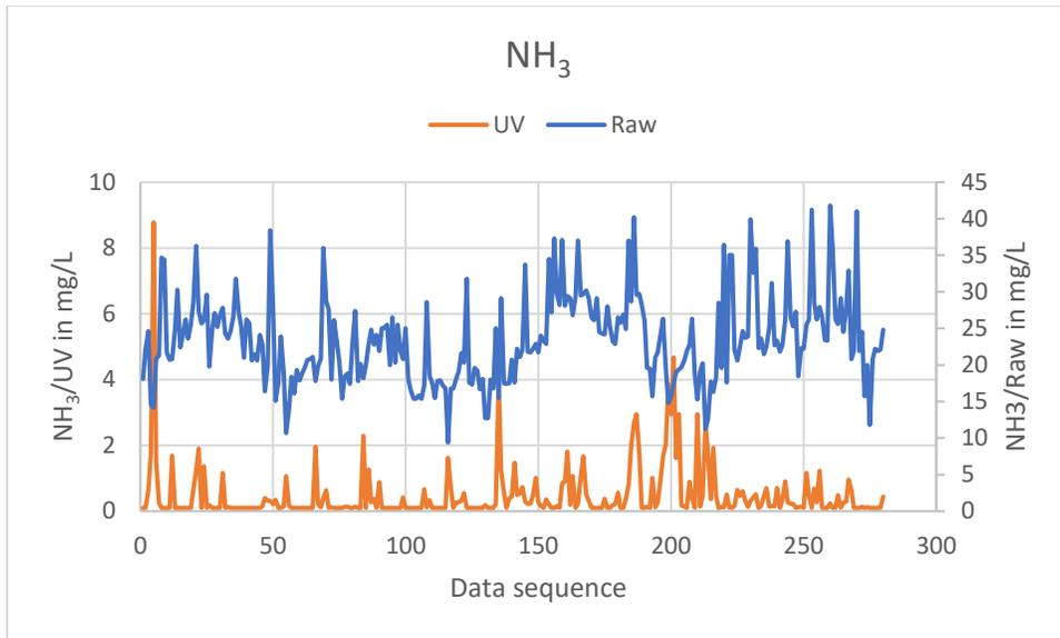
**Figure 3.7 Scatter plot of ammonia in the influent and effluent stream**
