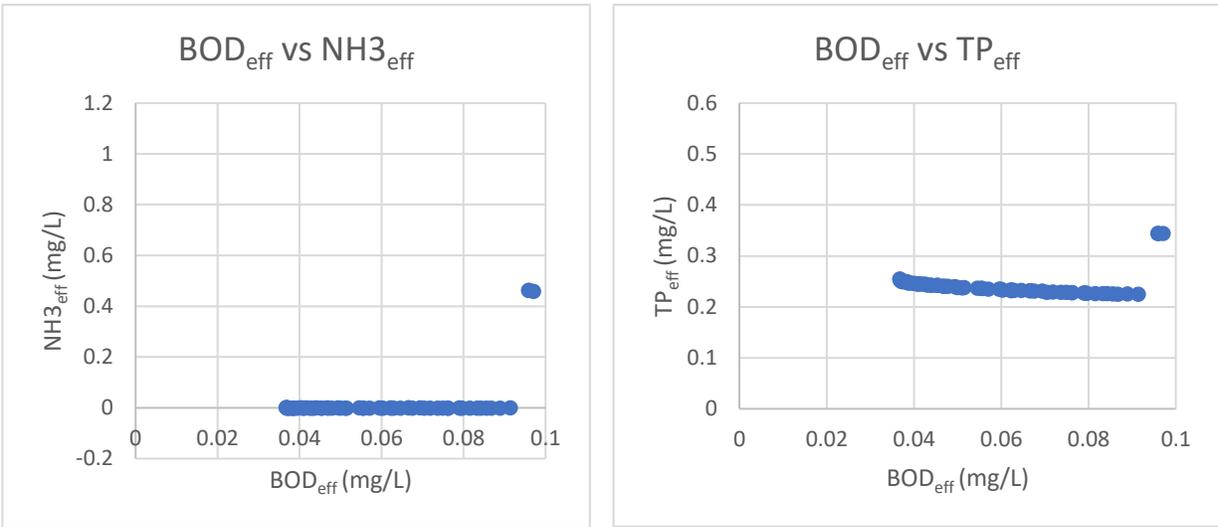
**Figure 5.14 Variation of  $\text{NH3}_{\text{eff}}$  and  $\text{TP}_{\text{eff}}$  with  $\text{BOD}_{\text{eff}}$  for case 2**
