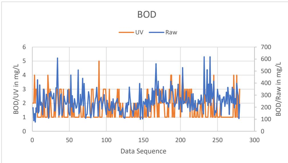
**Figure 3.4 Scatter plot of BOD in the influent and effluent stream**
