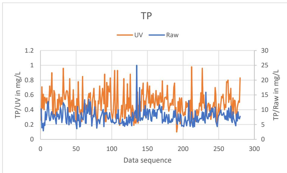
**Figure 3.6 Scatter plot of total phosphorous in the influent and effluent stream**
