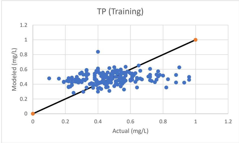
**Figure 4.5 Regression analysis of actual versus ANN-modeled TP concentration in effluent stream**
