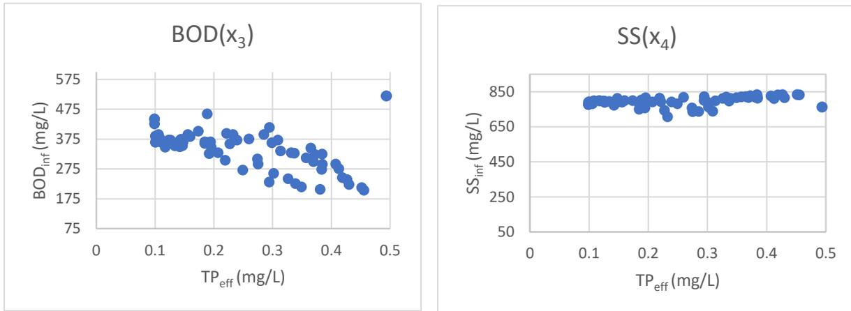
**Figure 5.24 Optimal variation of BOD<sub>inf</sub> and SS<sub>inf</sub> with TP<sub>eff</sub> for case 4**
