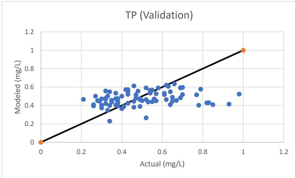
**Figure 4.12 Regression analysis of actual versus ANN-modeled TP concentration in the effluent stream**
