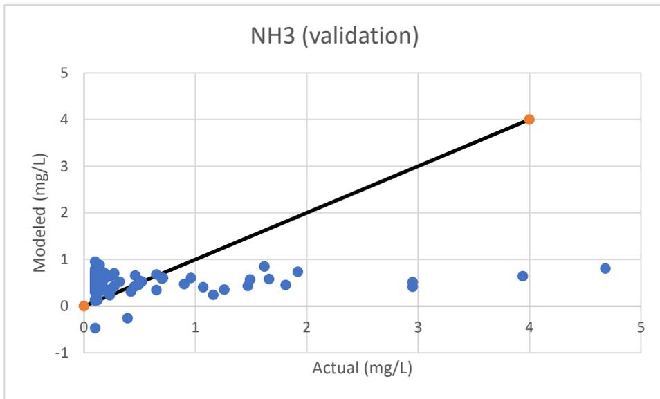
**Figure 4.13 Regression analysis of actual versus ANN-modeled NH3 concentration in the effluent stream**
