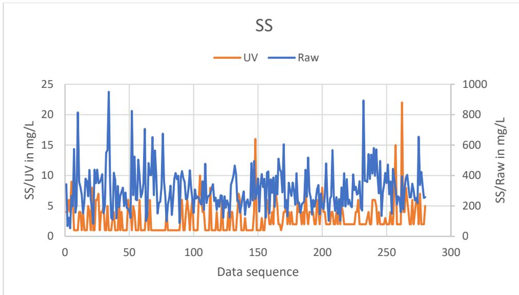
**Figure 3.5 Scatter plot of suspended solids in the influent and effluent stream**
