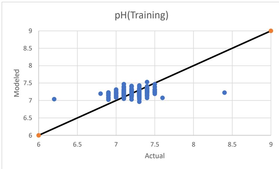
**Figure 4.7 Regression analysis of actual versus ANN-modeled pH values in effluent stream**
