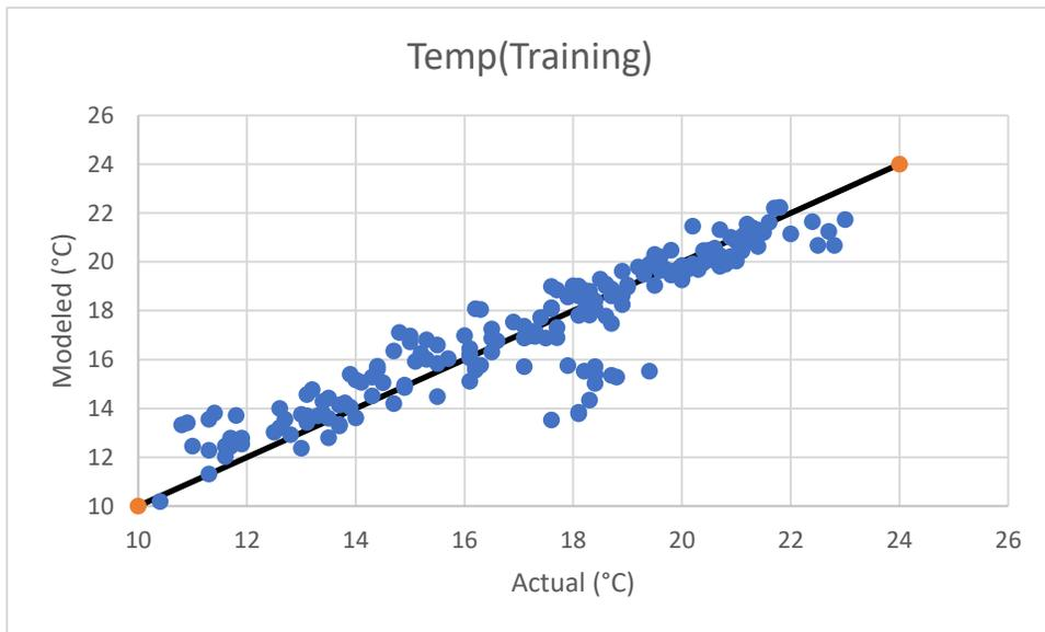
**Figure 4.9 Regression analysis of actual versus ANN-modeled temperature values in effluent stream**
