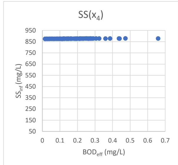
**Figure 5.5 Optimal variation of BOD<sub>inf</sub> and SS<sub>inf</sub> with BOD<sub>eff</sub> for case 1**
