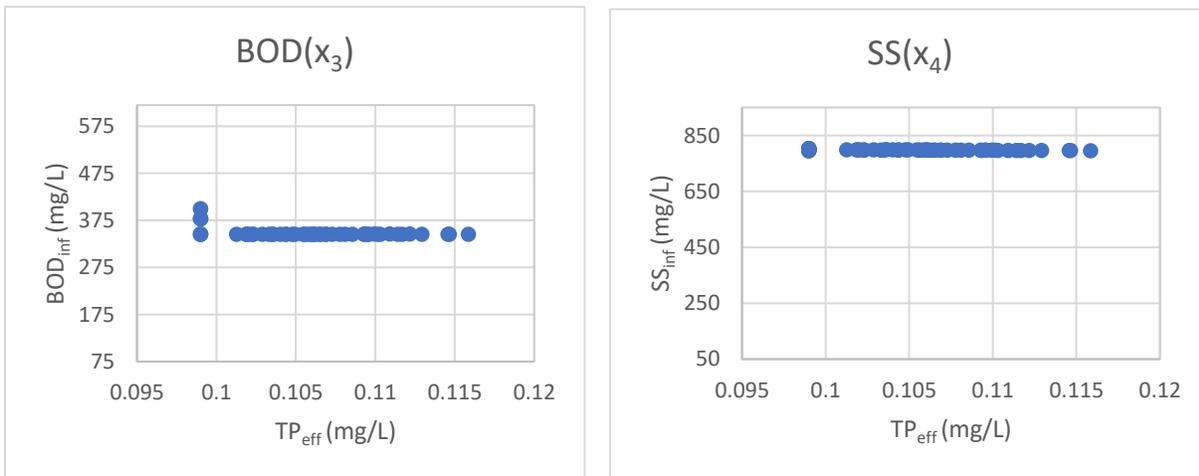
**Figure 5.17 Optimal variation of BOD<sub>inf</sub> and SS<sub>inf</sub> with TP<sub>eff</sub> for case 3**
