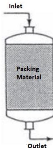
Figure 1.5 - Schematic of a simple packed bed device [16].
