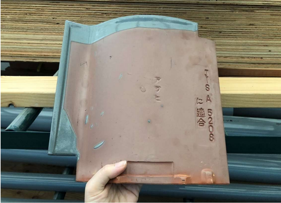
Figure 21 - Typical Japanese roof tile used to test the wind-borne debris impact resistance of the building envelope at DPRI, Kyoto University.
