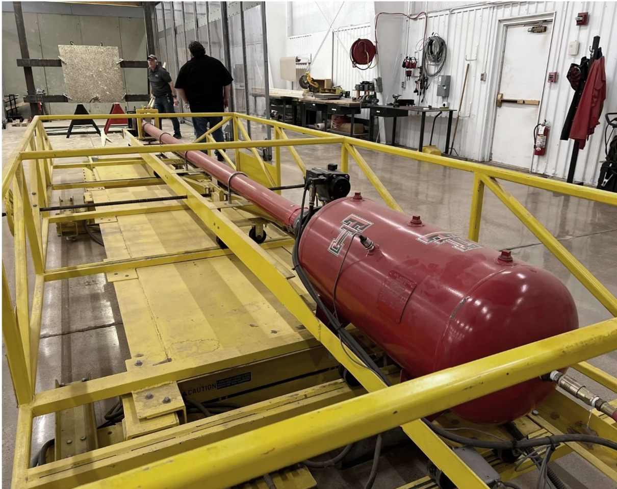
Figure 16 - Lubbock, Texas Tech University. Lumber projectile missile propulsion device (based on ASTM 2019). In the figure, the test specimen used to conduct the test is a concrete panel. Wind-borne debris impact test is used to test products that can be different from windows, doors, and curtain walling. The test goals are the assessments of the wind-borne debris impact performance of case study building technologies. The specimen area is surrounded by transparent vertical panels that are protecting who is attending the test from wood splinters.
