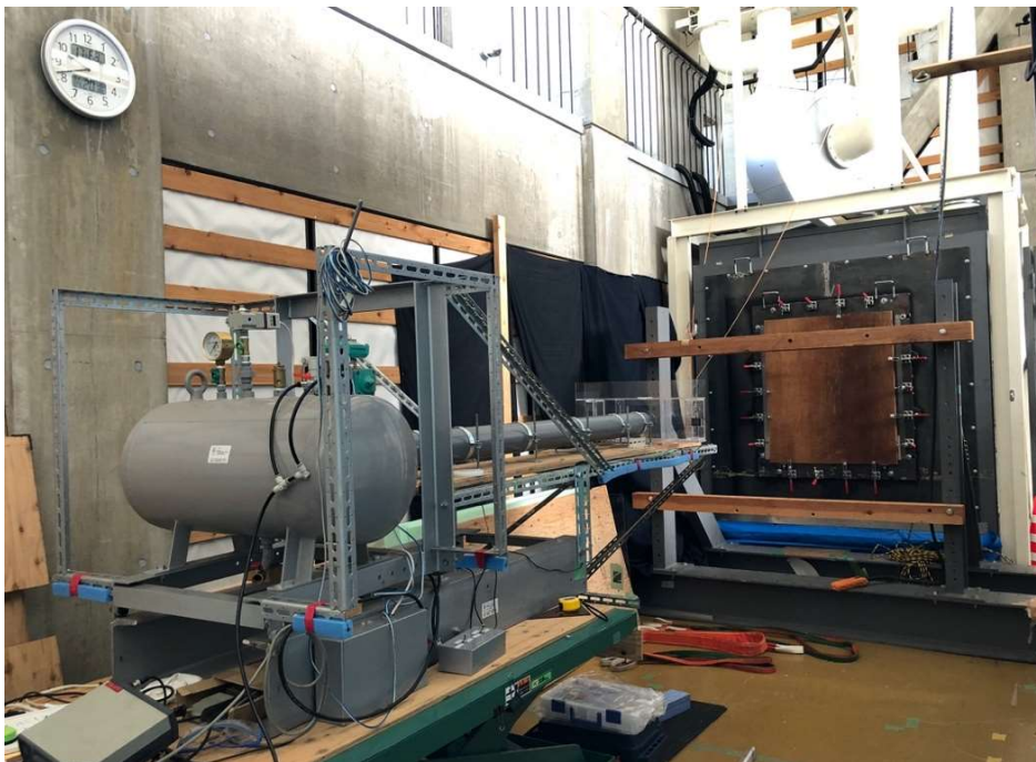
Figure 20 - Air cannon for missile impact-testing of glazing according to ISO 16932, DPRI, Kyoto University.
