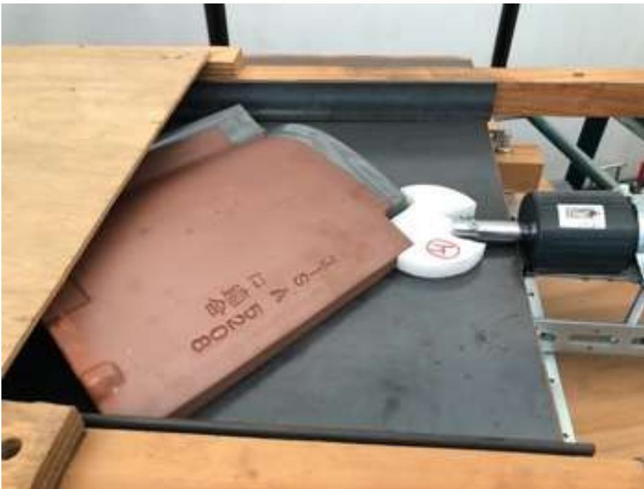
Figure 22 - Typical Japanese roof tile and air cannon adaptor equipment to shoot the tile through a glass sheet, DPRI, Kyoto University.
