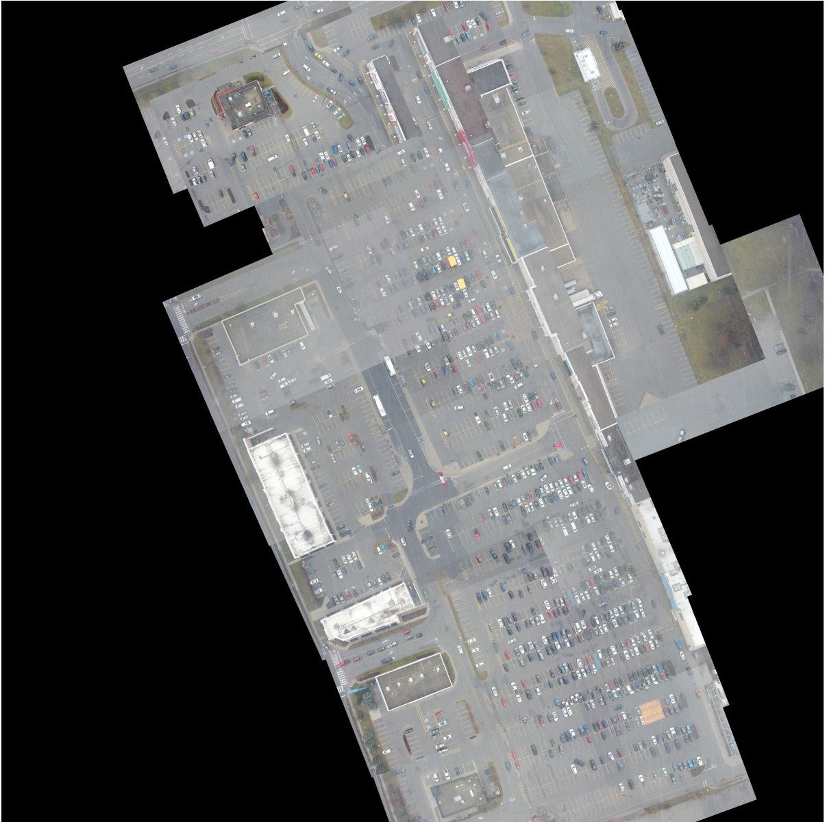
Figure 3.11: Subpar image stitching results obtained in case of large mosaic.
