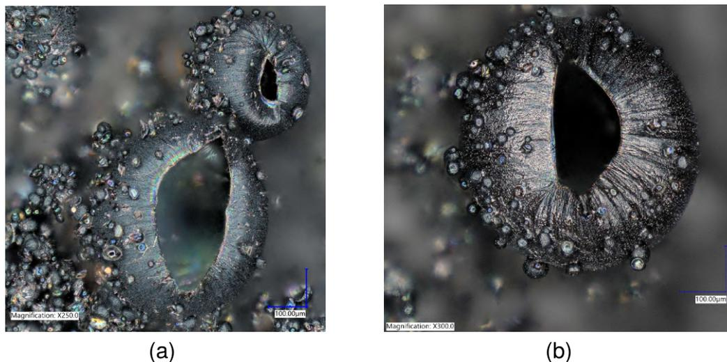
Figure 7.5: Optical microscopy images at (a) 250 $\times$  and (b) 300 $\times$ , demonstrate the hierarchical nature of microstructured polypyrrole films produced in the horizontal electrode configuration where stacked microspheres are observed at two distinct diameter ranges providing increased density of doping sites and capacity.
