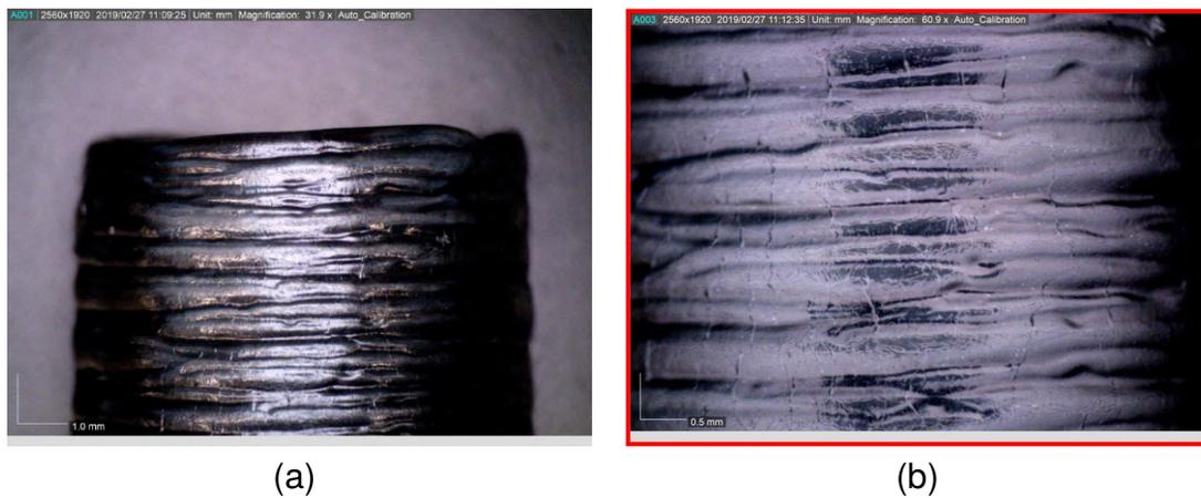
Figure 4.12: The spray coating of PEDOT:PSS onto a curved section of 3D DIW circular tube demonstrates a uniform coating accommodating both the curvature and surface roughness, however, PEDOT:PSS film cracking indicates the spray coating process requires further modification to produce thinner layers.
