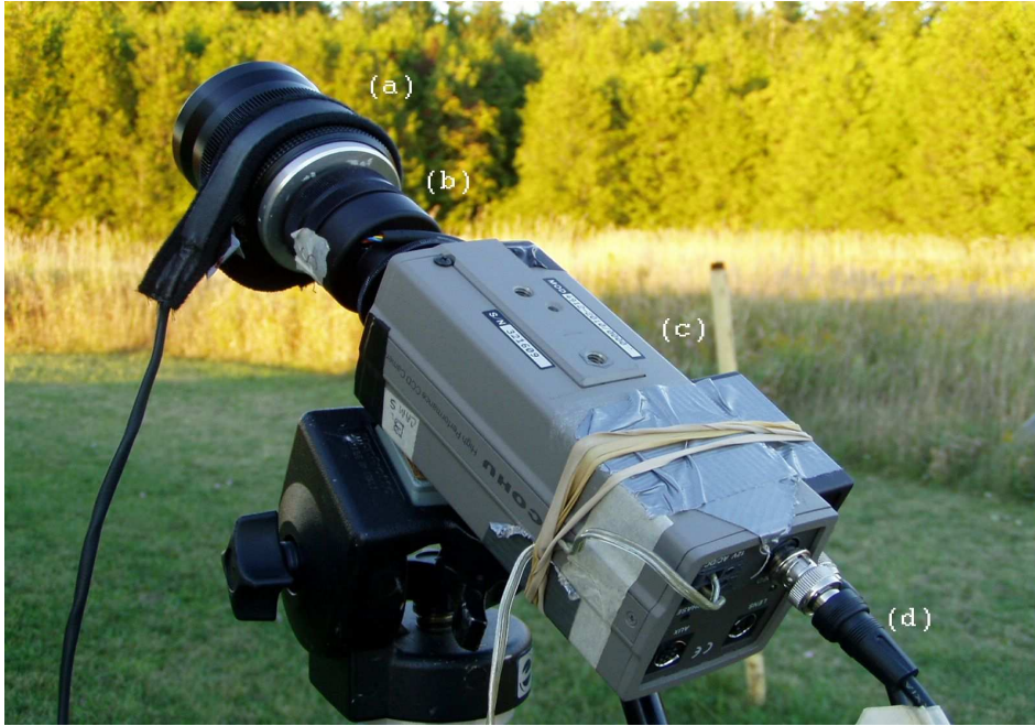
Figure 2.5: Component (a) 25 mm f/0.85 Fujinon objective, (b) Gen III Nitemate (380i), (c) Cohu 4910 CCD, (d) Analog CCD output to be digitized at the computer.
