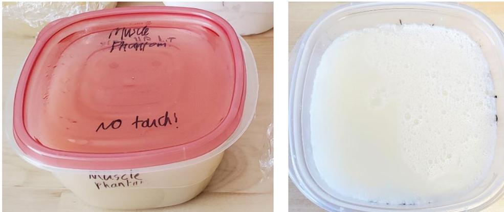
**Figure B.1:** Dielectric measurement setup showing the sample in the red Tupperware container (left) and the surface showing air bubbles (right).
