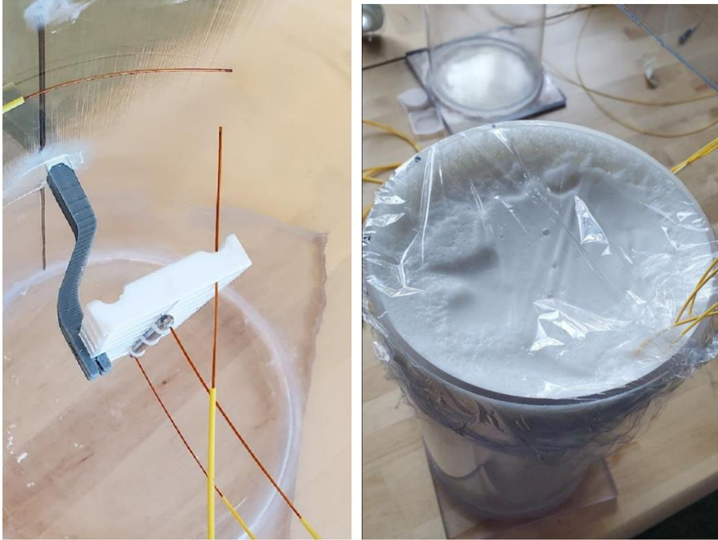
**Figure B.10:** **Left:** fiberoptic probes secured inside the phantom before pouring in the phantom material. **Right:** slight phantom shrinkage 24 hours after pouring was poured into a tupperware container to serve as our test sample that can undergo dielectric verification.
