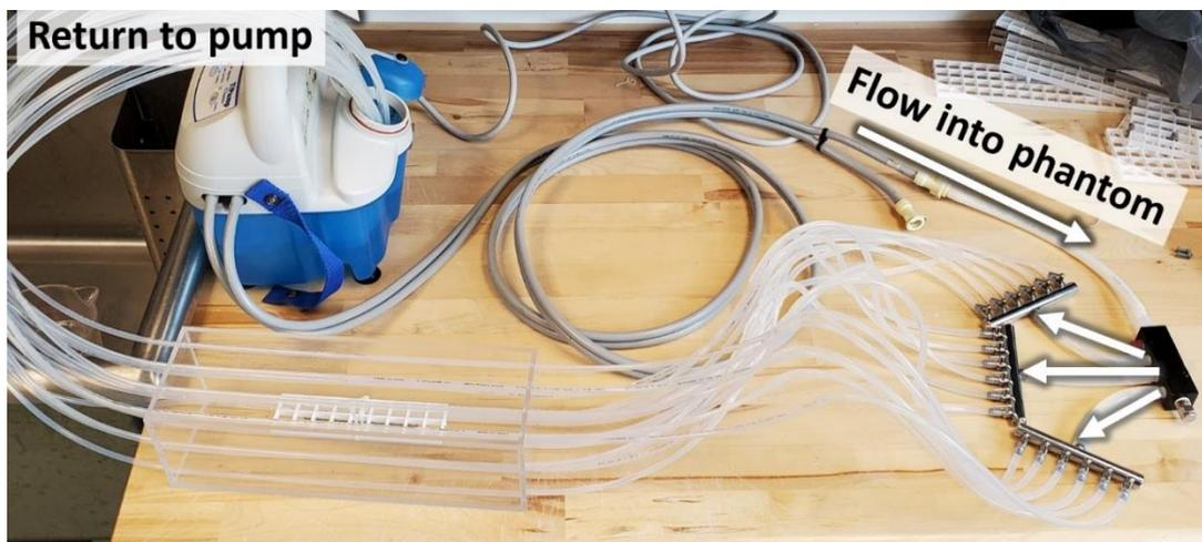
**Figure 3.2:** Initial setup to demonstrate the pumps' ability to provide sufficient flow to the perfusion phantom at the benchtop, prior to calibrating the flow in its final setup/configuration inside the RF exposure platform.
