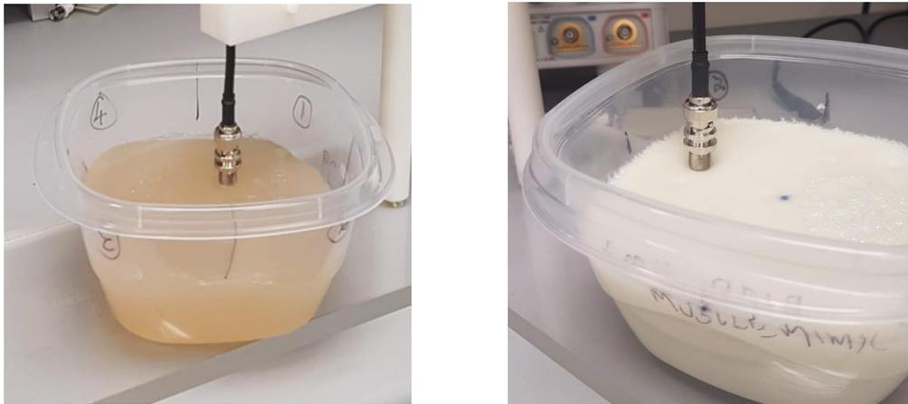
**Figure 2.5:** Okayama University muscle phantom (Left) and the Duke University muscle phantom (Right) undergoing dielectric characterization using the coaxial probe method
