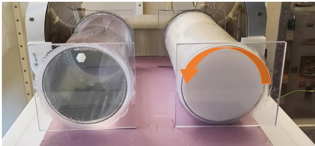
**Figure 2.18:** Cylinder phantoms filled with saline (left) and muscle mimicking material (right) in their testing configuration. The arrow shows how the muscle phantom was rotated 180 degrees during the calibration, but then returned to its original position for testing.
