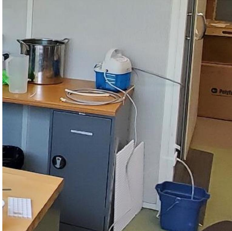
**Figure 3.5:** Pump positioning outside the Faraday cage, showing the inlet tubing in grey (near the pump) and the bucket that the phantom drains into (bottom).
