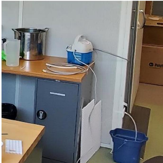
**Figure E.4:** Pump positioning outside the Faraday cage, showing the inlet tubing in grey (near the pump) and the bucket that the phantom drains into (bottom).
