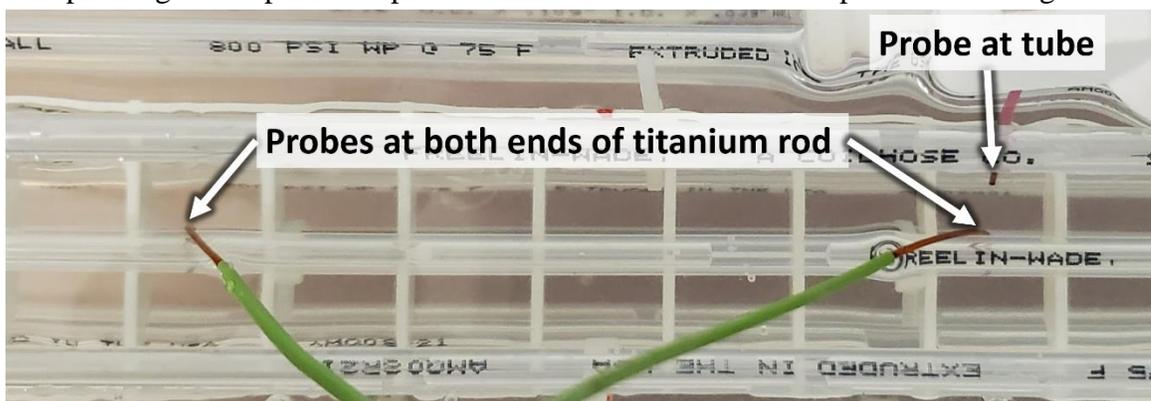
**Figure 3.8:** Fiberoptic probe placement showing the two probes at either end of the titanium rod, and the probe place on the tube directly adjacent to the edge of the rod. Heating the titanium rod in the HEC gel tends to generate the most heating around the ends, and thus the probe on the tube is the shortest distance from the titanium rod.
