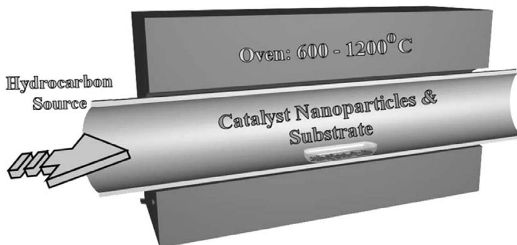
Figure 2.18 Schematic diagram of a thermal CVD setup.
