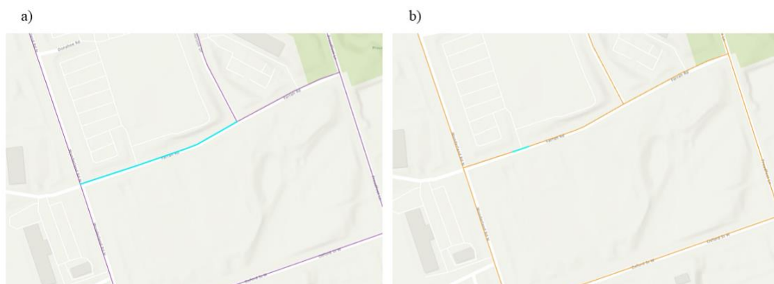
Figure 2-3: a) Example of a 247.5m segment (Farrah Road) highlighted in light blue and b) One of ten 24.75m lixels along a Farrah Road segment highlighted in light blue.
