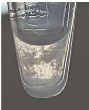
**Figure 4.12.** *Photograph of  $6.6 \mu\text{M}$  NISTmAb in an Eppendorf vial after 10 min at  $95 \text{ }^\circ\text{C}$ , pH 6.32. The presence of aggregated protein (white amorphous precipitate) is readily apparent.*
