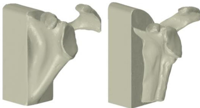
Figure 4.1: Models of the Normal (left) and B2 (right) Sawbone Scapulae [129].
