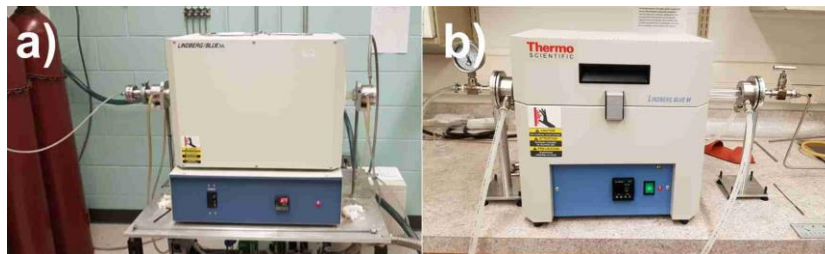
Figure 2.3. a) Lindberg/Blue M 1500°C single zone furnace. b) Lindberg Blue Mini-mite 1100°C single zone furnace.
