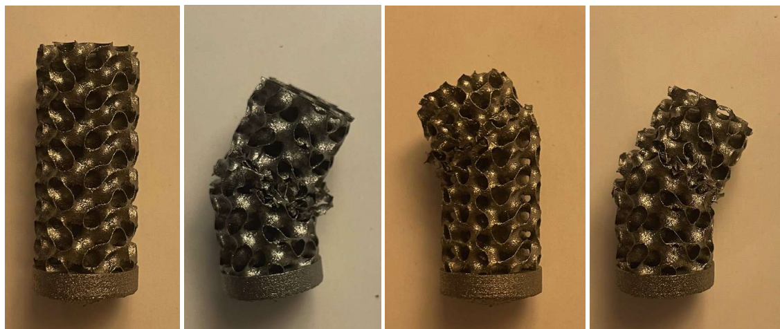
Figure 5-15. 90P specimens after fatigue testing. From left to right, specimens were tested at a maximum applied load of 50%, 70%, 80%, and 90% of their yield force.
