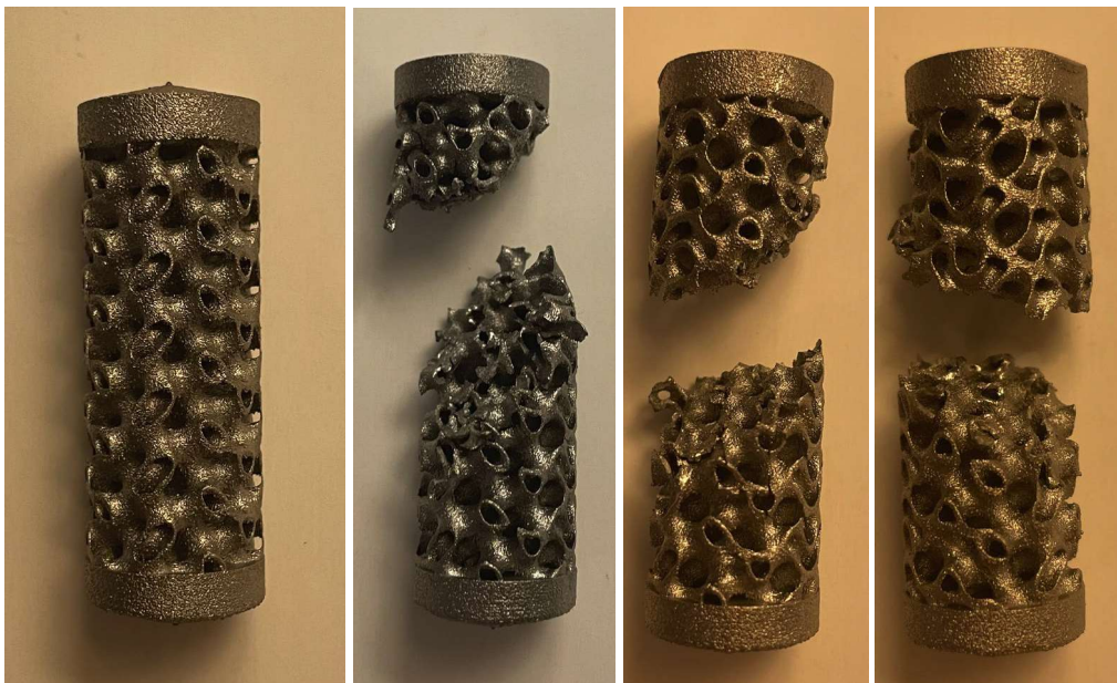
Figure 5-12. 70P specimens after fatigue testing. From left to right, specimens were tested at a maximum applied load of 50%, 65%, 70%, and 75% of their yield force.
