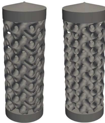
Figure 2-2. CAD models of the gyroid cylinders with end caps developed for the experimental testing. Left: 60P. Right: 90P.
