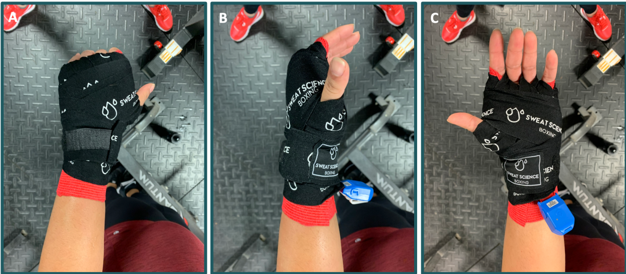
Figure 3.5. Left hand of an athlete demonstrating placement of linear wraps over sensors. A. Dorsal side of hand. B. Radial side of hand. C. Palmar side of hand.
