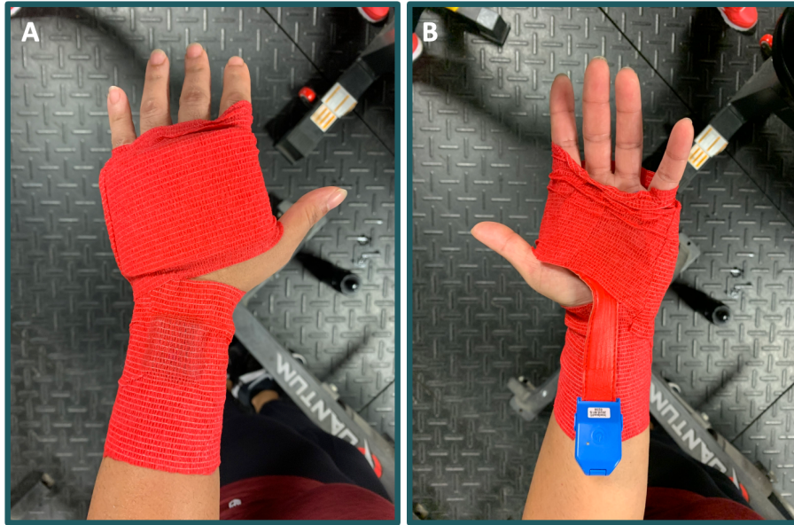
Figure 3.8. Left hand of an athlete demonstrating maintenance of placement of novel loadpad and StrikeTec sensors held with self-adhesive wrap after completing striking protocol. A. Dorsal side of hand. B. Palmar side of hand.
