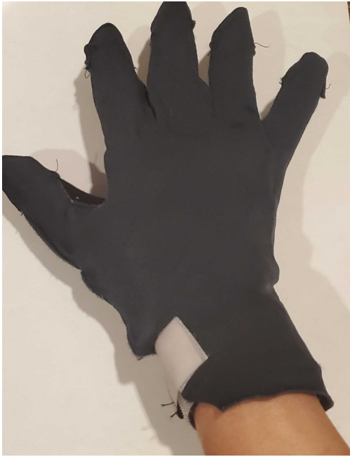
Figure 3.9: Dorsal view of polyester blend fabric on the glove that goes over and sticks to the base layer Velcro glove and cover the hardware.
