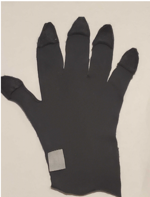
Figure 3.8: The polyester blend fabric that goes over and sticks to the base layer Velcro glove and cover the hardware.
