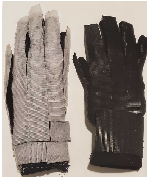
Figure 3.6: The two different glove (base layer) sizes that the hardware attach to with Velcro.
