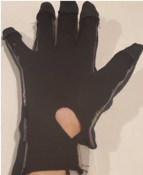
Figure 3.10: Palmar view of polyester blend fabric on the glove that goes over and sticks to the base layer Velcro glove and cover the hardware.
