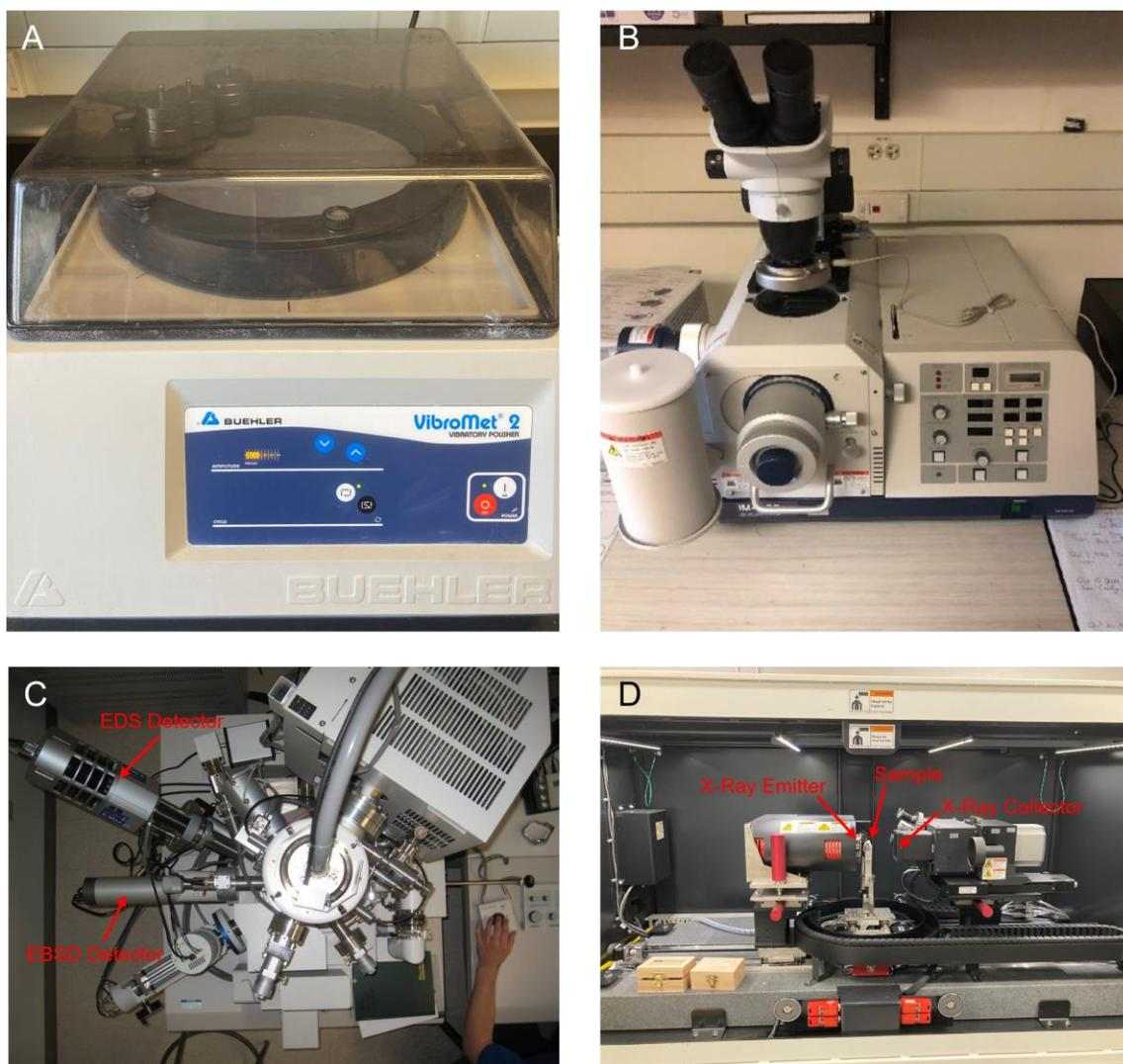
**Figure 5: A) Vibromet Vibratory polisher. B) Hitachi 4000 Argon Ion Mill. C) The Hitachi SU6600 variable pressure Field Emission Gun Scanning Electron Microscope. Arrows indicate the attached energy dispersive X-ray detector and electron backscatter diffraction detector. D) The interior of the Zeiss Xradia 410 Versa from Surface Science Western. Arrows indicate the X-ray emitter, the sample in the sample holder, and the X-ray collector.**
