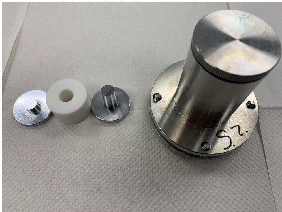
**Figure 3.14** A model cell with the internal parts and the shell
