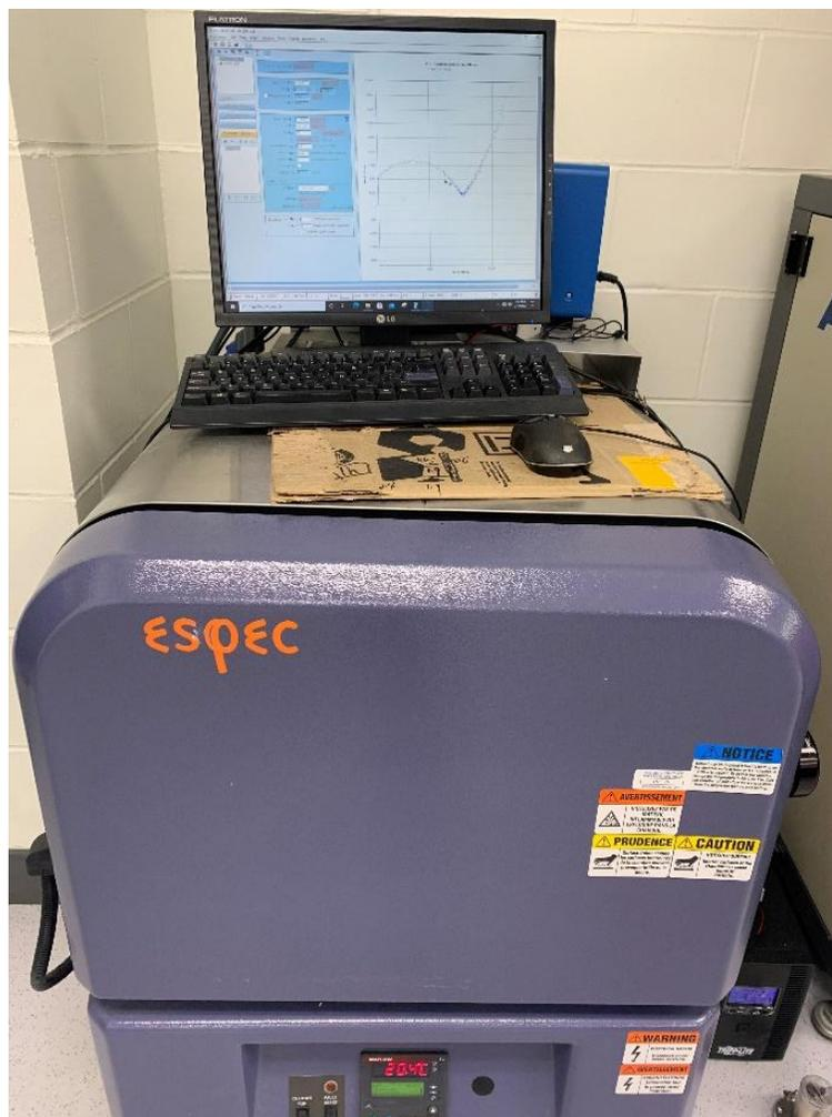
**Figure 3.15** The VMP3 working station with a programmable thermal chamber.
