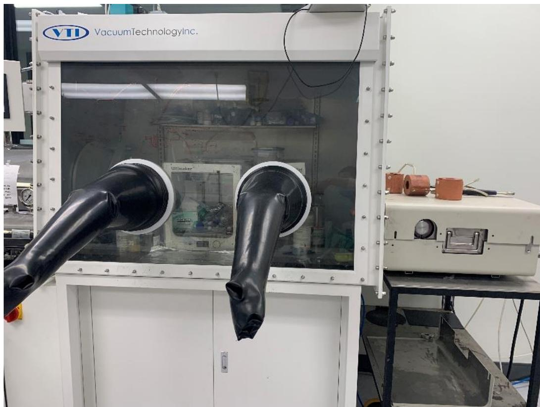
**Figure 3.3** The Gemstar-8 ALD system as well as the connected glove box.
