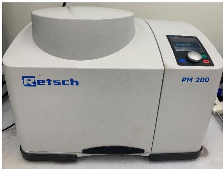
**Figure 3.1** PM200 two-station planetary ball mill produced by Retsch
