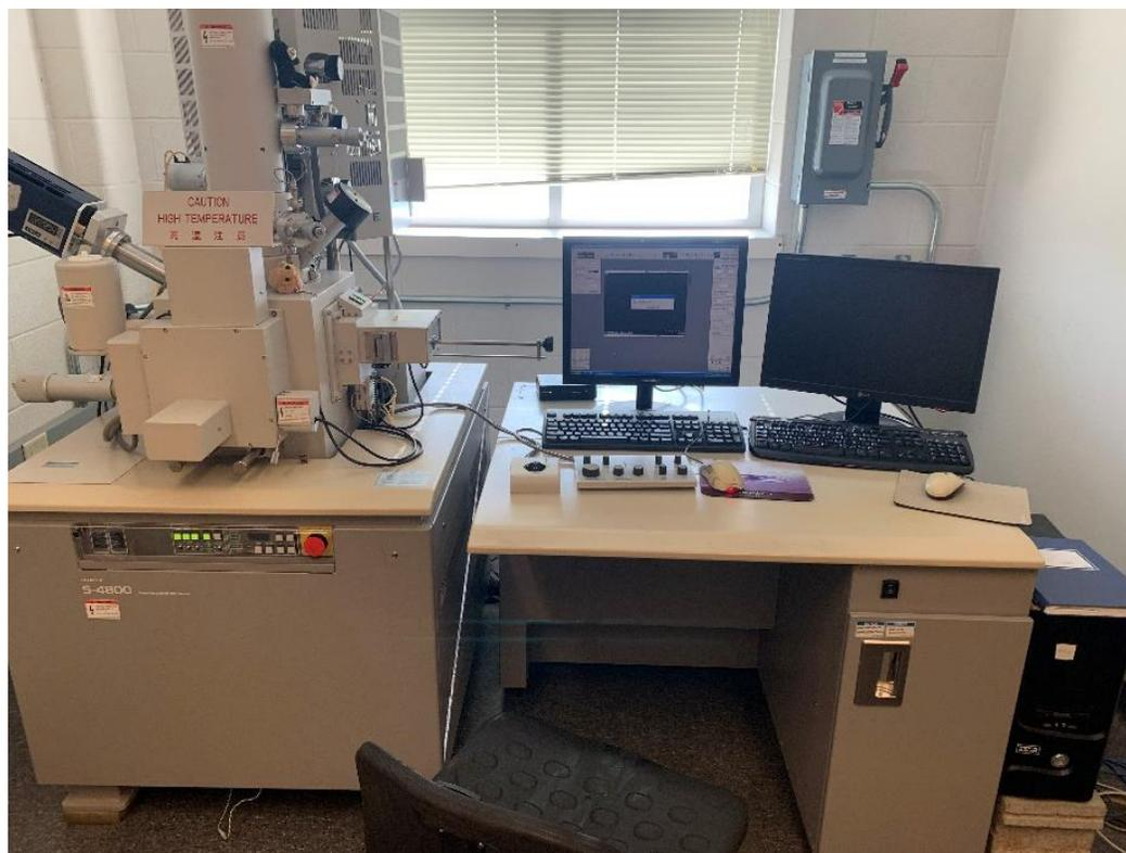
**Figure 3.4** The Hitachi S-4800 SEM, equid with EDS.
