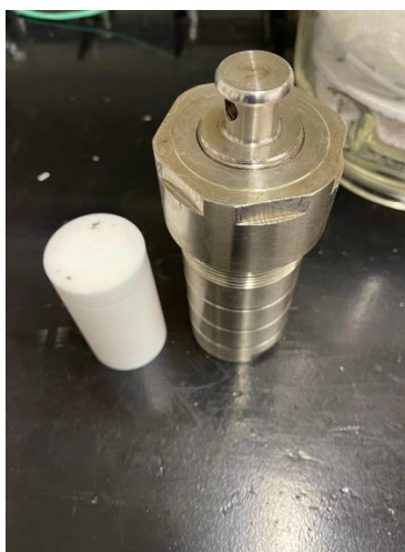
Figure 2- 5. Hydrothermal synthesis autoclave reactor with polytetrafluoroethylene (PTFE) lined vessel.
