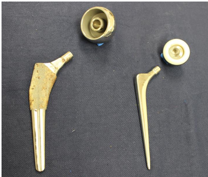
Figure 9: (left) Hemiarthroplasty device utilising a large head, (right) hemiarthroplasty device utilizing a head within a head with a polyethylene liner between.
