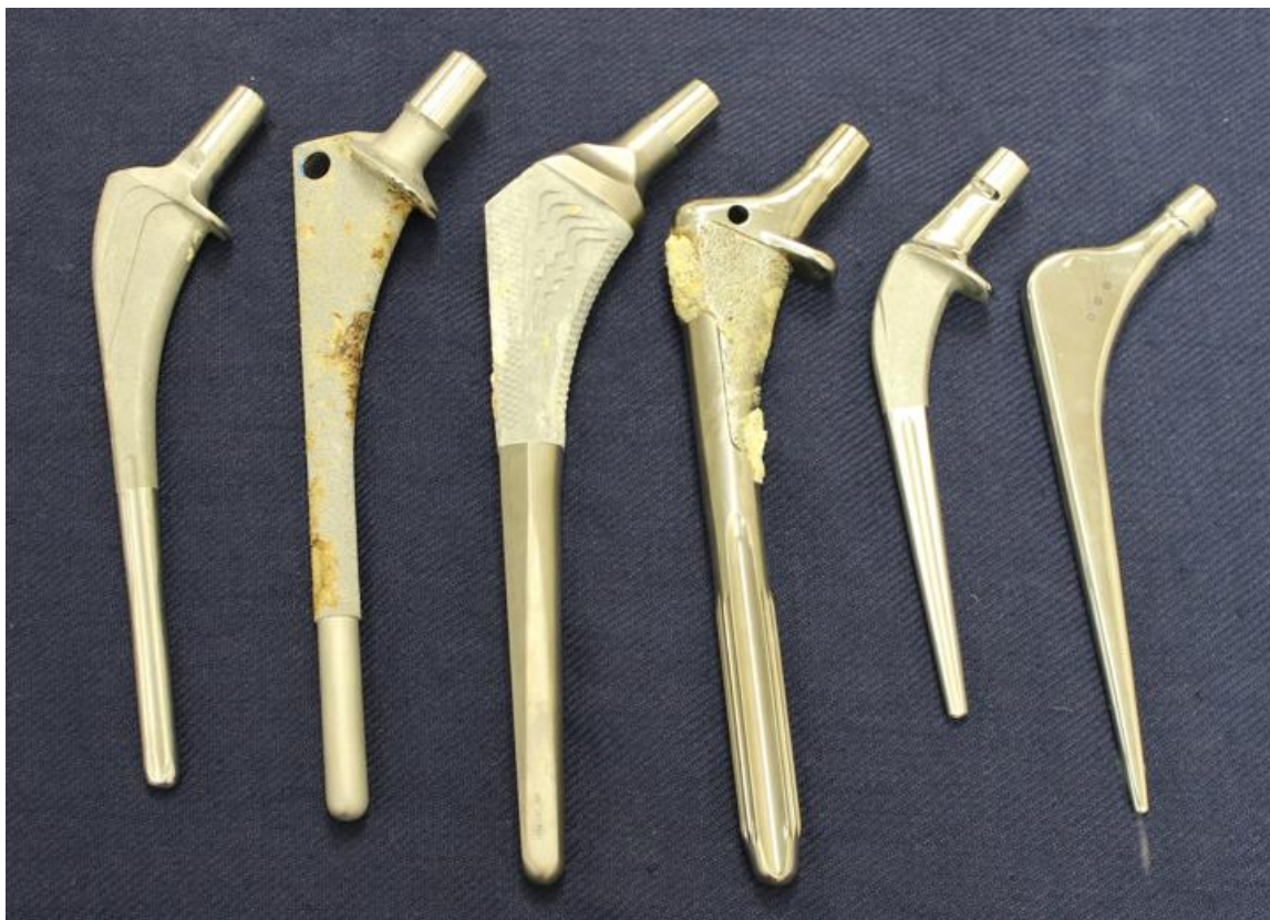
Figure 5: A variety of available stems, showcasing major design differences in the distal stem component of the device.
