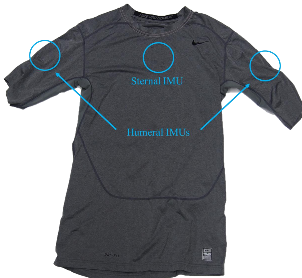
Figure 3-3: Custom motion capture (MOCAP) shirt with pockets shown for the sternal and humeral inertial measurement units (IMUs)
