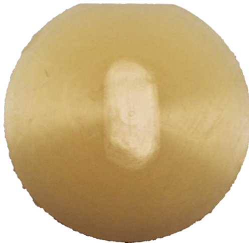
Figure 2-4: Wear scar on VEXLPE plate
