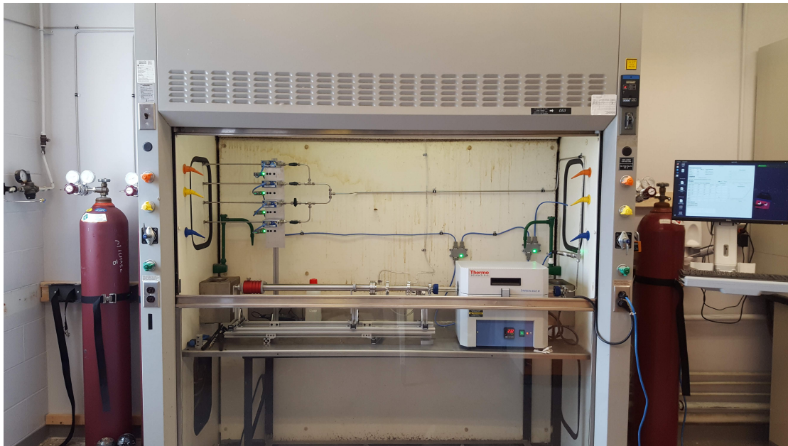
Figure C.1: Photograph of the assembled CVD system. The system fits into a fumehood and is controlled from the computer on the right.
