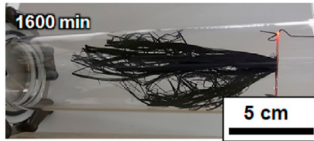
Figure 2.6: From Sugime et al. [62]. 14 cm long CNTs grown using a cold-gas CVD process with in situ supplementation of iron and aluminum.
