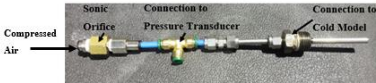
Figure 2-17. Device used for pressure measurement with backflushing.
