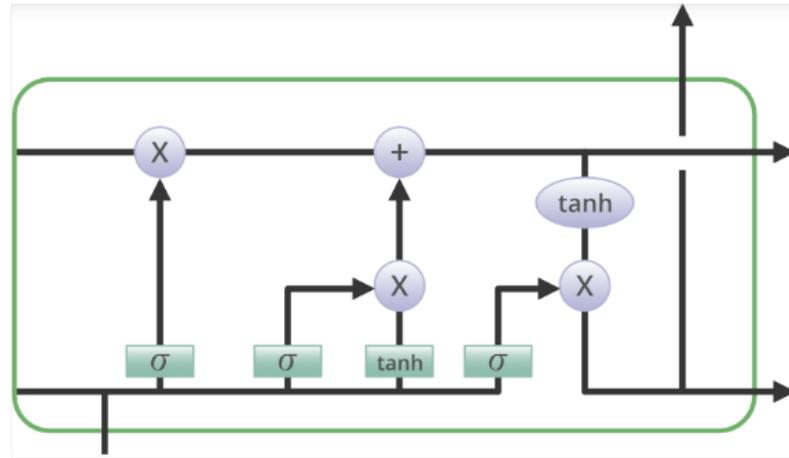
**Figure 2.19: LSTM full architecture [49].**
