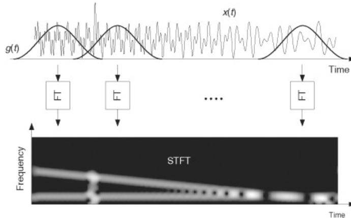
**Figure 2.6: Illustration of STFT by taking Fourier transforms of a windowed signal [5].**
