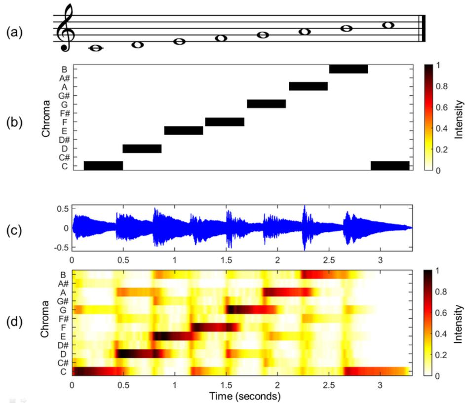
**Figure 2.10: (a) The musical score for the C-major scale. (b) Produced chromagram from the musical score. (c) A piano recording of the C-major scale. (d) Audio recording generated chromagram [2].**
