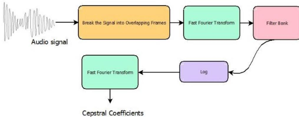
**Figure 2.9: Flow diagram of MFCC [22].**
