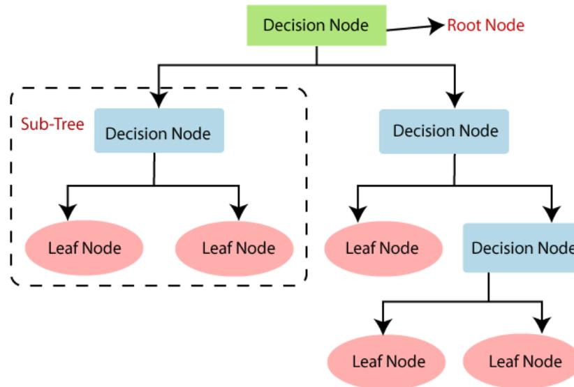
**Figure 2.13: Decision Tree Algorithm workflow diagram [29].**
