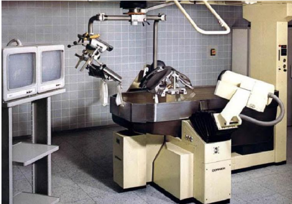
Figure 1: The Dornier HM3 lithotripter and a patient being prepared for treatment in the Dornier HM3. Source: Dornier Medtech
