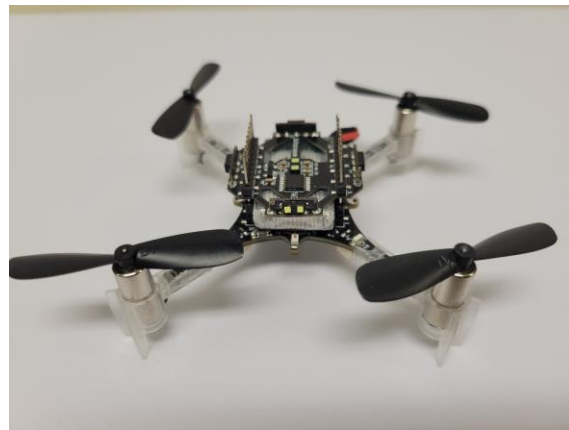
Figure 21 Image of Crazyflie 2.1 with 6 mounted LIDAR sensors and a downward facing optical flow sensor
