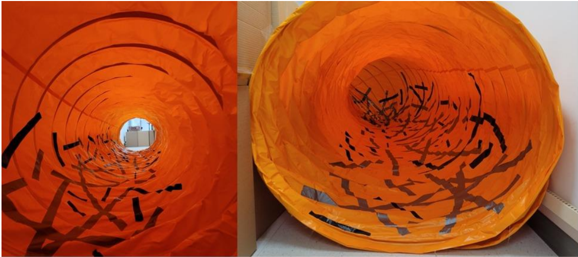
Figure 22 Pipe testing environment. The entrance to the pipe as seen from inside and outside of the pipe. The diameter of the pipe is 100cm and the length is 700cms. A 90-degree bend occurs 600cms into the Pipe
