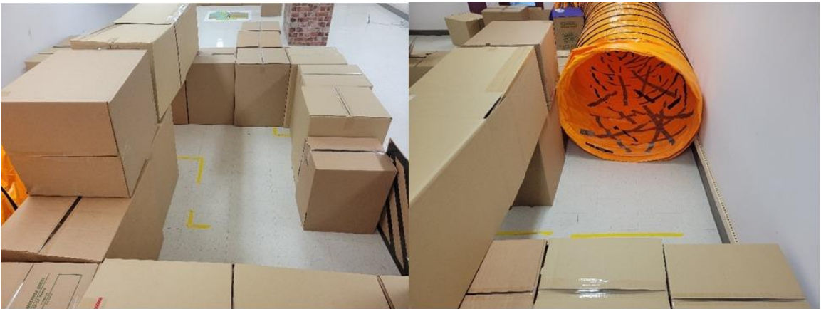
Figure 23 The Beginning section of the combined test bed. On the left the space where the drone is deployed. The right image shows the entrance into the pipe.
