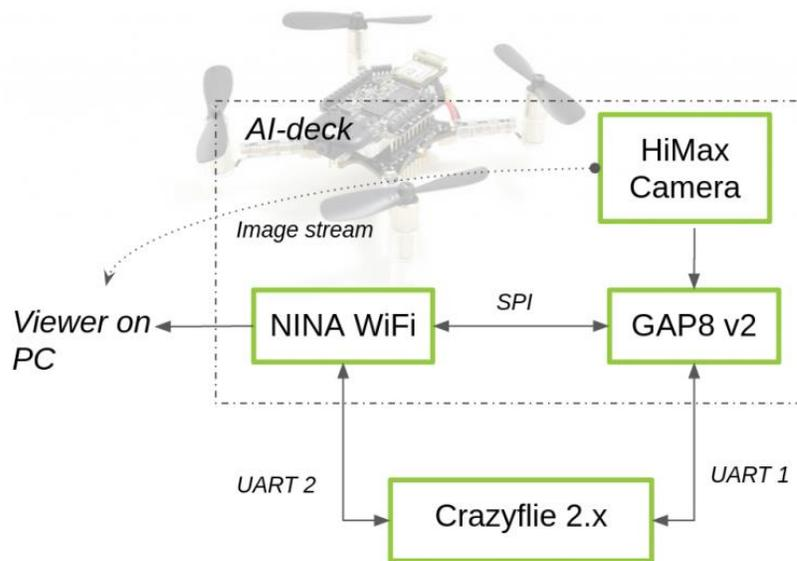
**Figure 14: AI-deck system architecture [61]**
