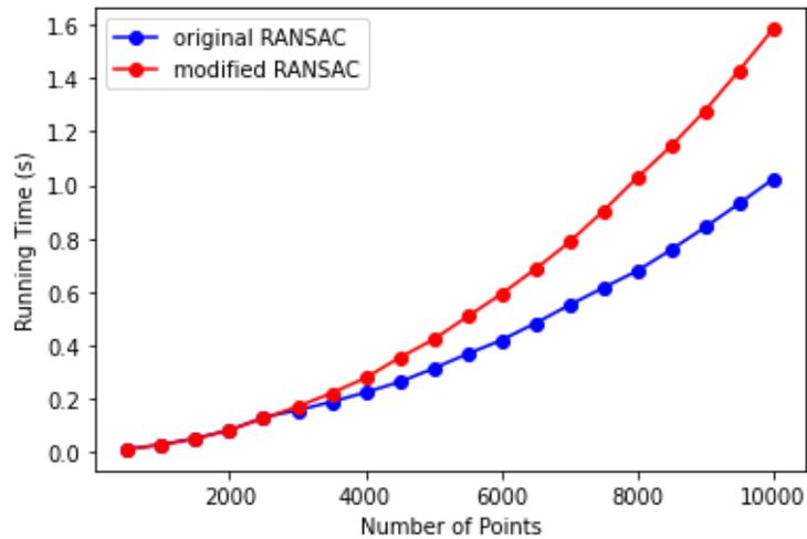
**Figure 21: The relationship between the number of points and the running time when  $\sigma = 10$**
