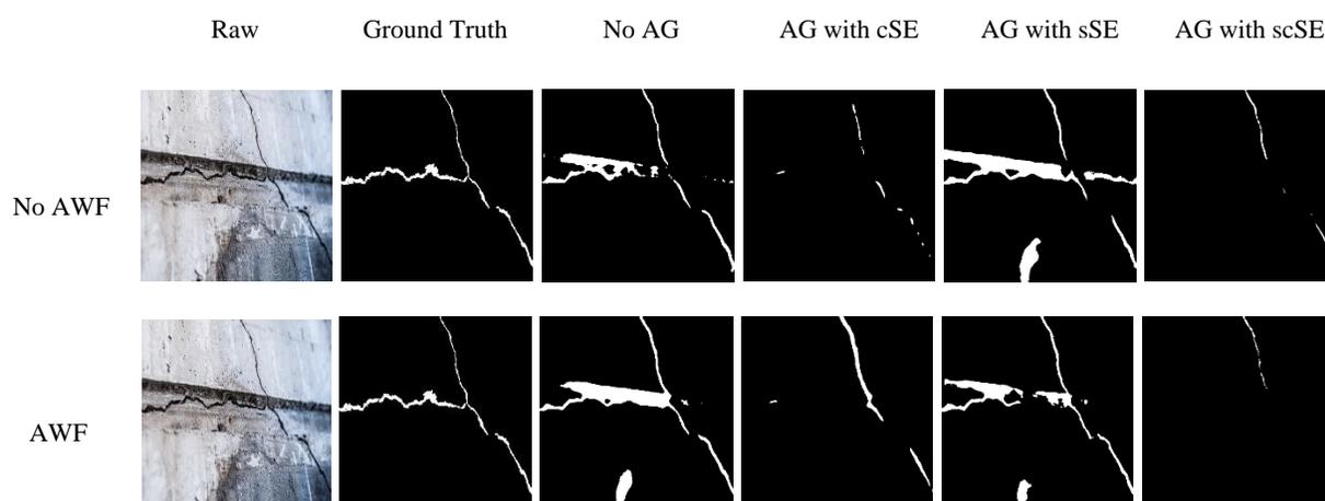
**Figure 41: The image, ground truth, and corresponding predicted label maps of each model version on the merged dataset**
