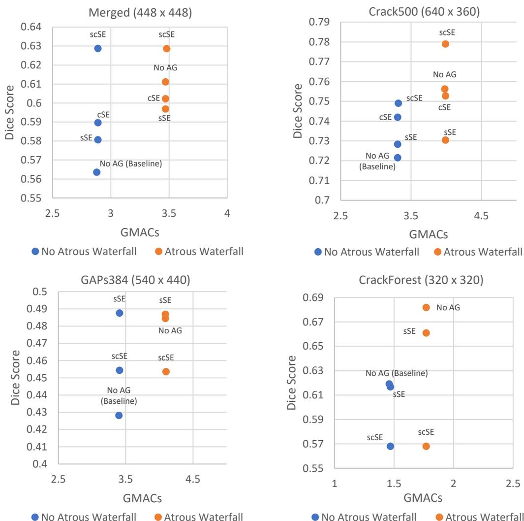
**Figure 46: The effect of adding the atrous waterfall block and using different attention gates on the dice score and number of computations (GMACs)**
