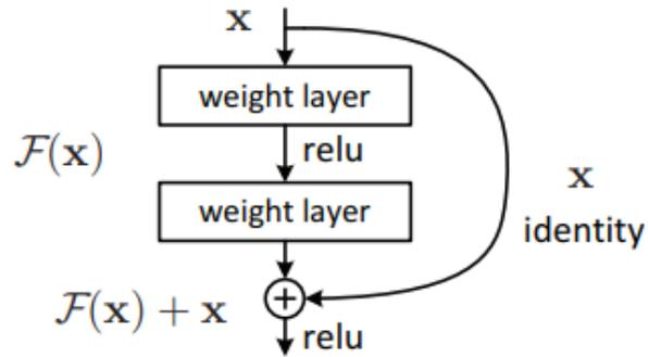
**Figure 4: Residual block in ResNet [28]**
