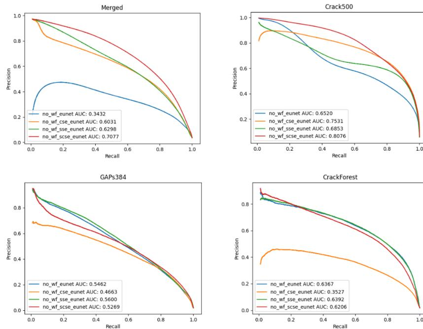
**Figure 39: The Precision-Recall Curves (PRC) and corresponding AUPRC scores for the Efficient U-Net models without the atrous waterfall block**
