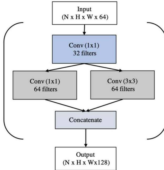
**Figure 11: A fire module used in Squeeze U-Net [45]**
