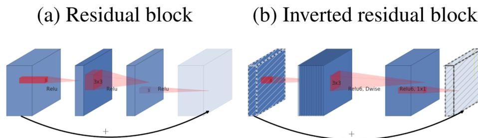
**Figure 29: The architecture of (a) a residual block and (b) an inverted residual block [68]**
