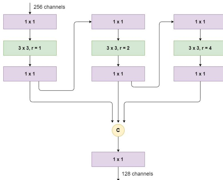
**Figure 35: Atrous Waterfall Block included in the bottleneck layer of Efficient U-Net. A feature map of 256 channels is taken in as input and the final  $1 \times 1$  convolution reduces the output channel space to 128 channels**
