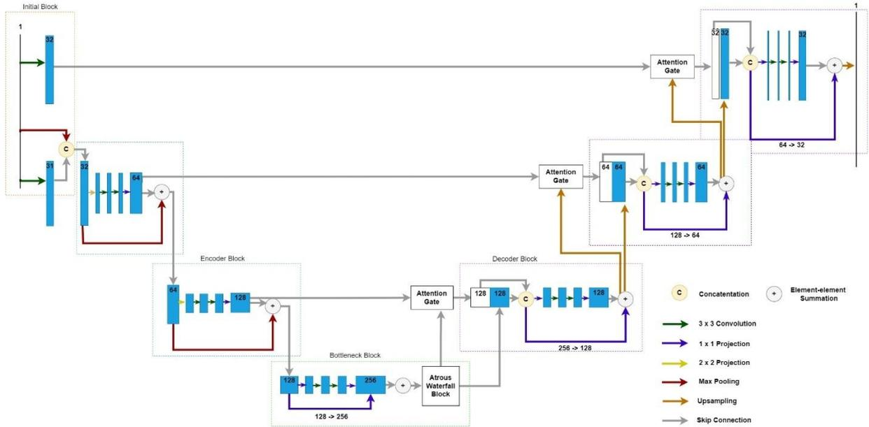
**Figure 33: Proposed Efficient U-Net Architecture. Blue blocks represent feature maps, with the width denoting feature space and height denoting resolution**
