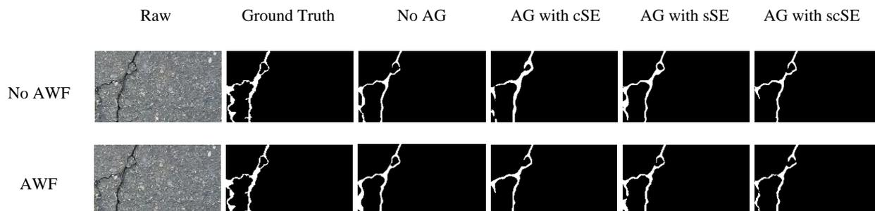
**Figure 42: The image, ground truth, and corresponding predicted label maps of each model version on the Crack500 dataset**
