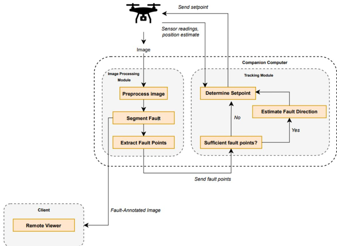
**Figure 12: High-Level Proposed System Architecture**
