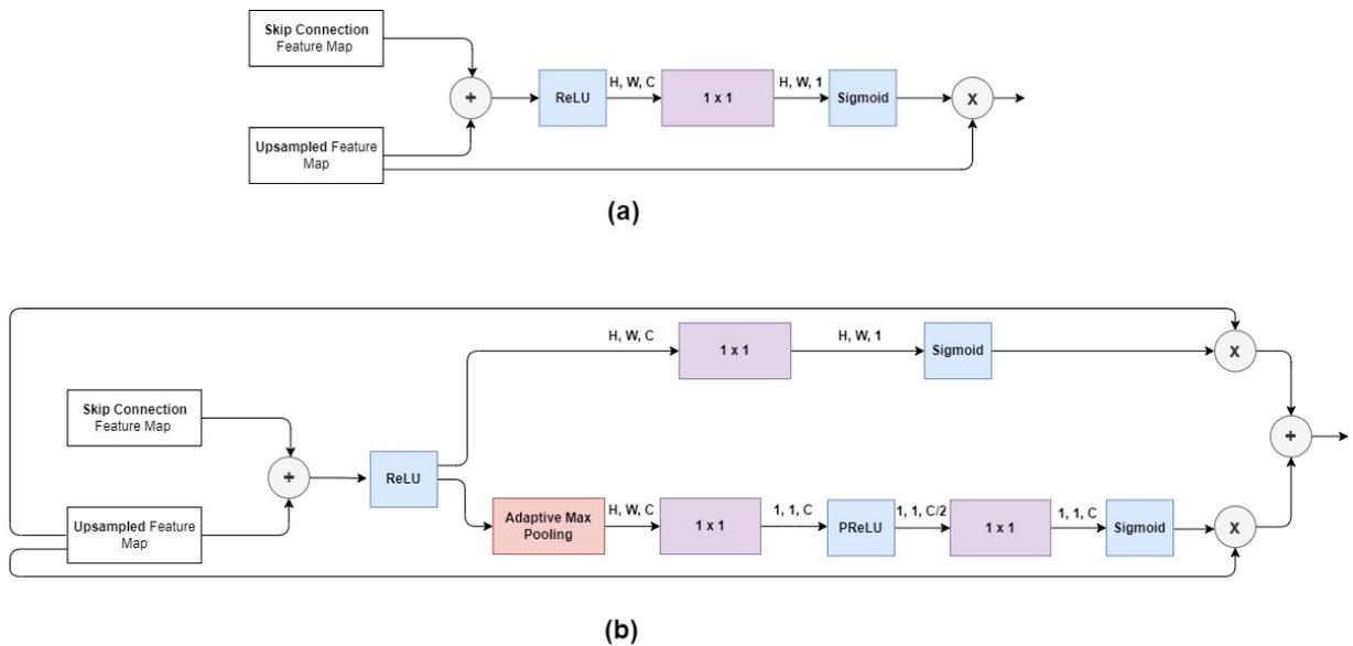
**Figure 37: Implemented SE block variants in the decoder block of the network: (a) sSE block; (b) scSE block**
