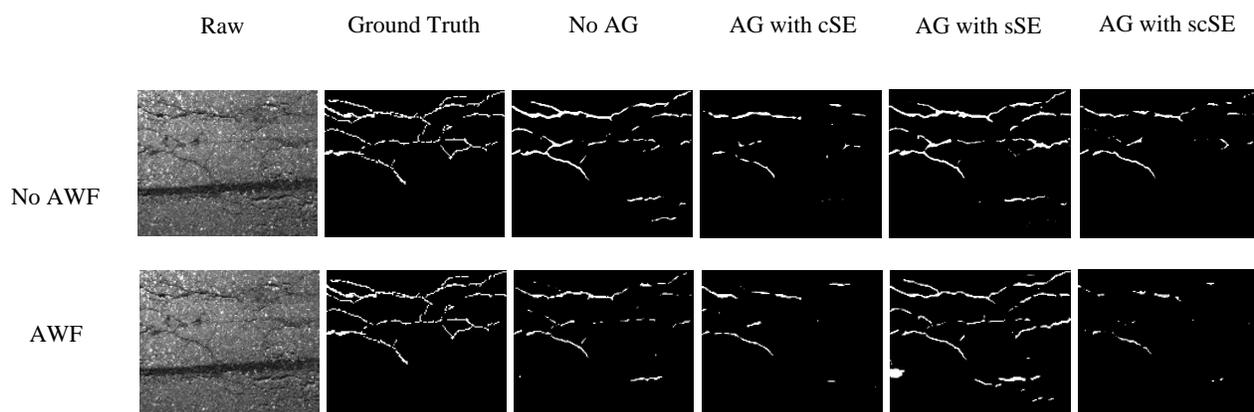
**Figure 43: The image, ground truth, and corresponding predicted label maps of each model version on the GAPs384 dataset**
