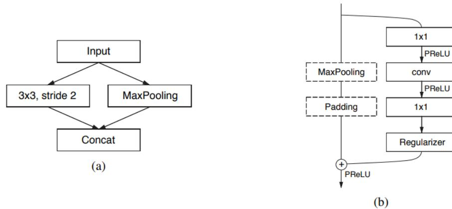
**Figure 25: (a) ENet initial block; (b) ENet down-sampling bottleneck block [63]**
