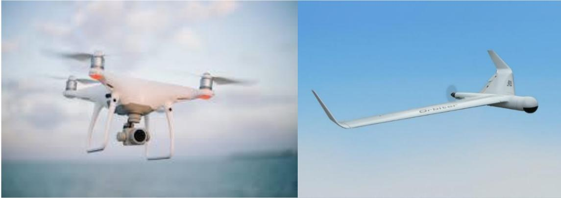
**Figure 5: Left – rotary-wing drone [89]; right – fixed-wing drone [90]**
