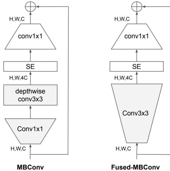
**Figure 32: The differences between an MBConv and Fused-MBConv block [70]**
