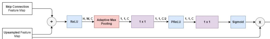
**Figure 36: Attention Gate in Efficient U-Net**
