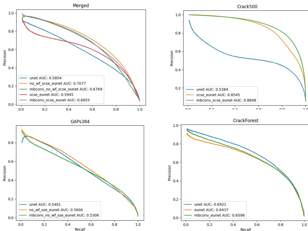
**Figure 47: The Precision-Recall Curves (PRC) and corresponding AUPRC scores for the U-Net (baseline), Efficient U-Net, and MBConv Efficient U-Net models**
