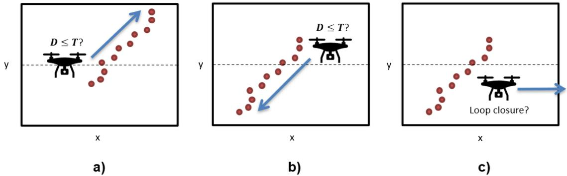
**Figure 18: Mapping extracted fault points to  $x, y$  coordinate view frame: (a) more points in the mapped to the upper half of the view frame; (b) more points in the mapped to the lower half of the view frame; (c) loop closure detected**
