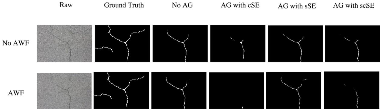
**Figure 44: The image, ground truth, and corresponding predicted label maps of each model version on the CrackForest dataset**
