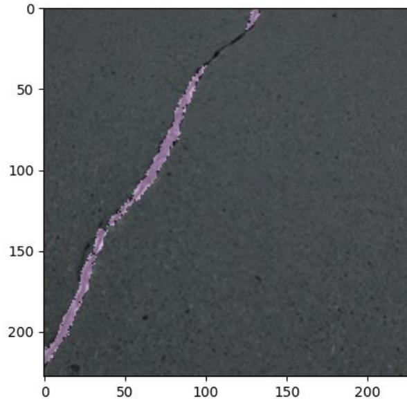
**Figure 7: Output of an FCN used for semantic segmentation of cracks**
