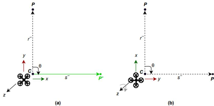
**Figure 15: (a) Changing the drone direction of motion; (b) rotating the drone**
