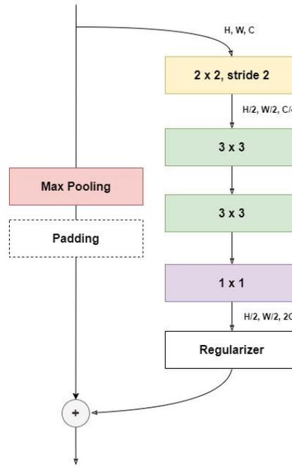
**Figure 34: Encoder block in Efficient U-Net**
