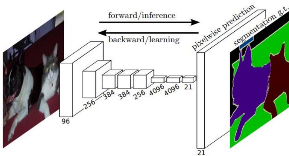
**Figure 3: FCN performing semantic segmentation. The number of channels (feature space size) produced by each convolutional layer is indicated [42]**
