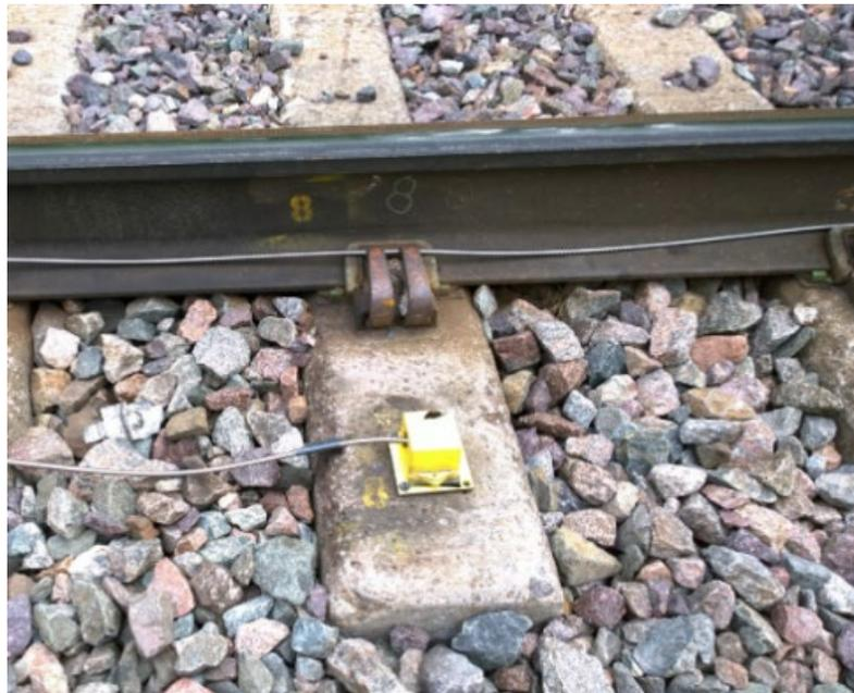
**Fig. 4.2 Cross-tie mounted accelerometer**
