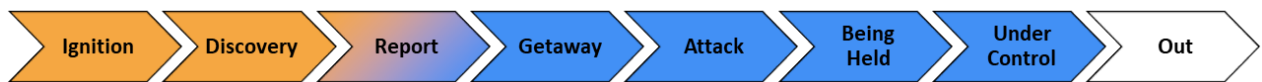
Figure 3.3: Visual representation of fire lifetime events, along with the detection phase (orange) and the action phase (blue).
