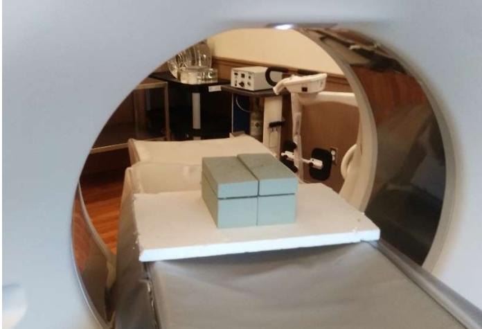
Figure F.1. Set-up of 45 teeth in florist foam inside the clinical CT scan at St-Joseph's hospital, London, Ontario. Picture taken by Émy Roberge.
