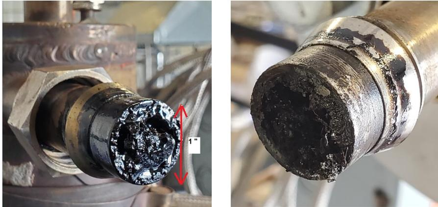
**Figure 5-4 Tar accumulated in the reactor-cyclone connection**
