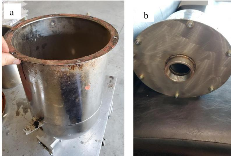
Figure 5-3 a- un-sealed hopper b- sealed hopper cap and mounted with valve
