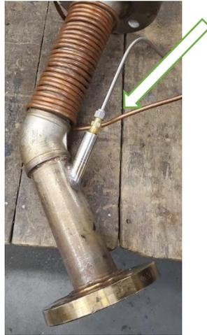
**Figure 5-2 New manufactured inlet to blow any residue after the experiment, or continuously supply inert gas (N<sub>2</sub>)**
