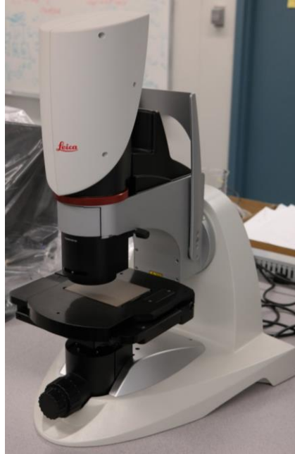
Figure 3-3: Leica DVM6A digital microscope used for optical microscopy. Photo copied from RAMPS group website ( https://www.rampsgroup.org/members ), Photo taken by Giles Whitaker.
