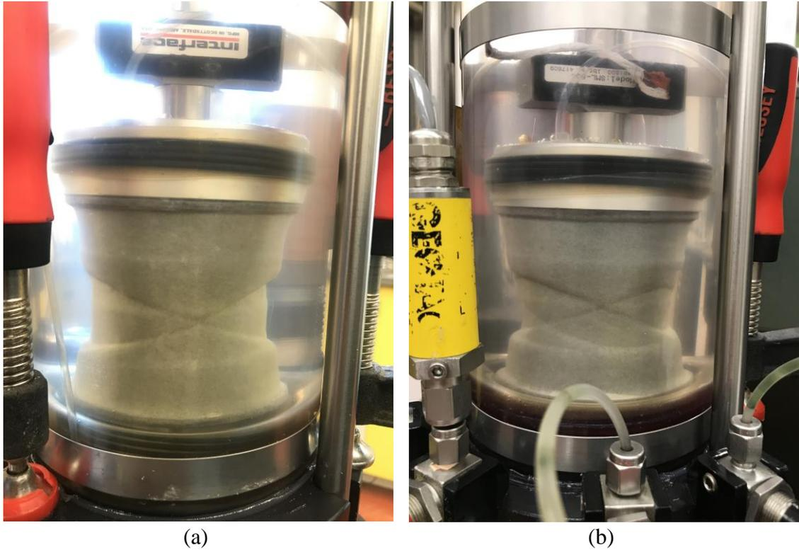
**Figure 2-8:** Formation of shear bands in EKEU tests at  $p'_c$  of (a) 335 kPa and (b) 117 kPa
